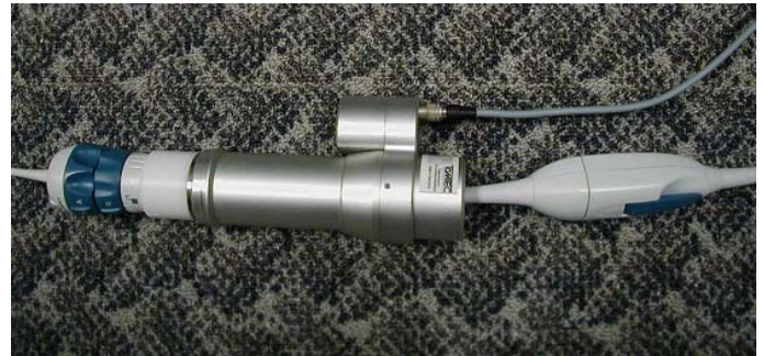
Figure 11. A 10F AcuNav catheter shown with rotation hardware (Tomtec Imaging Systems, Unterschleissheim, Germany) attached to the catheter steering mechanism.
