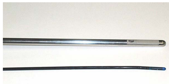
Figure 1. Rigid 24 Fr. AcuNav prototype (top) compared to one of the current products, a 10 Fr. version.
