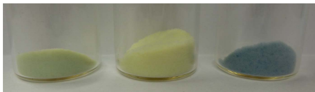
Figure 5: Color change of MO7:Pd before (b) and after (c) the exposure to 20 ppm ethylene. After the gasochromic reaction, the probe was rinsed with synthetic air for another 20 minutes, to reach the original state again (a). The measurement was performed in synthetic air with 40% r.H.
