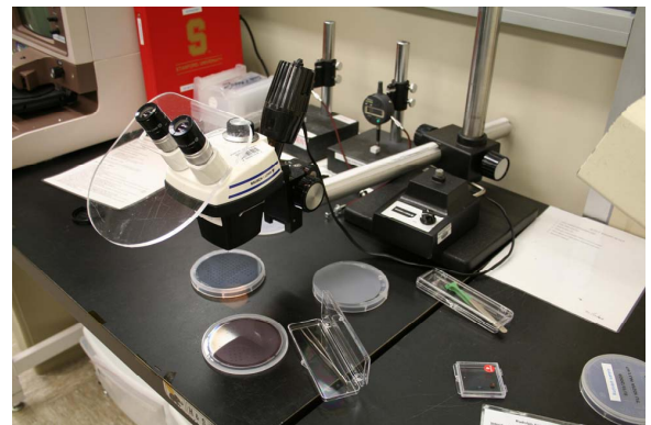
Figure 7: Assembly experiment setup, with microscope and assorted tweezers for chip placement.
