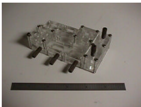
Figure 7. Microfluidic motherboard with attached modules.
