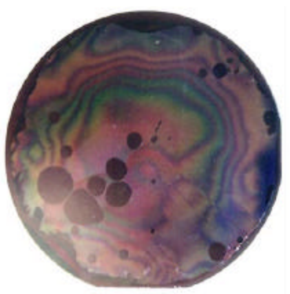
Fig. 4. Photograph of a 3C-SiC/SiO 2 /Si substrate.
