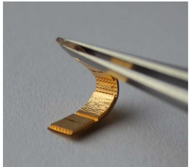
Figure 4: Demonstration of flexibility and gold plating quality.
