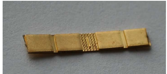
Figure 3: Photo of the Au coated OSTE polymer device.
