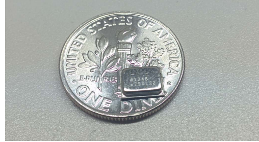
Fig. 1: Photo of a packaged MEMS gyroscope (4×6×1 mm 2 ) used as a test vehicle for virtual rotation demonstration.
