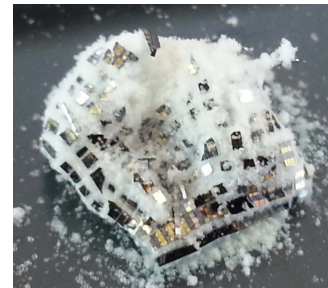
Figure 9: Chip transience is achieved via constrained expansion of the microparticles. The typical result is a heap consisting of a mixture of particles and silicon dust.
