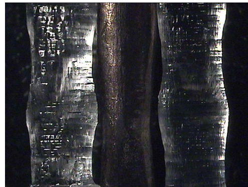
Figure 1: Optical photograph of the real seal whisker (center) and the artificial whisker (left and right) fabricated in this work.
