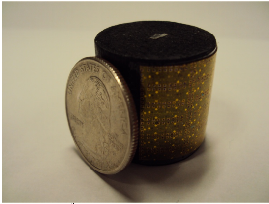
Fig. 4: A 2 \times 2 \text{ cm}^2 piece of flexible substrate containing an array of 75 pressure sensors.
