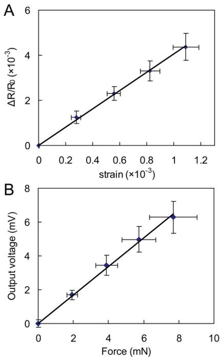
Figure 4: Calibration of the paper-based force sensor. (A) Calibration plot of the relative resistance change vs. the applied mechanical strain ( $N=7$ ). (B) Calibration plot of the circuit voltage output vs. the applied force ( $N=7$ ).
