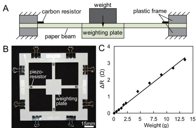
Figure 6: A paper-based weighing balance. (A) Schematic side view and (B) photograph (top view) of the device. (C) Calibration plot of the resistance change from one sensing beam vs. applied weight.
