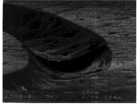
Figure 10: SEM picture of 3D microstructure created in PTFE surface.
