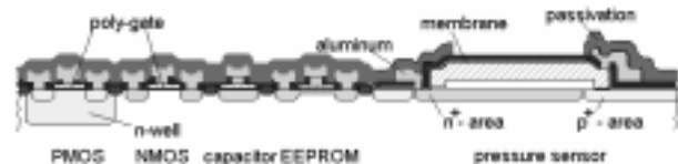
Figure 1: Cross-section of a monolithic integrated pressure sensor device.
