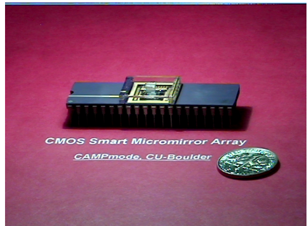
Figure 12. The final device packaged in a 40 pin DIP package.
