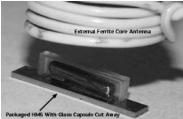
Figure 10: Glass-silicon package with HMS enclosed.
