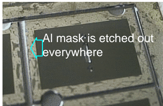
(a) 130^\circ\text{C} baked negative resist created many cracks after ICP-RIE then Al mask beneath have been etched.
