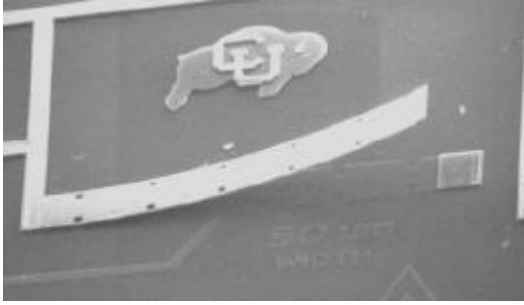
Figure 3: Micrograph of Microconnector. Deflection Occurs Naturally Due to Residual Stress Within the Beam.
