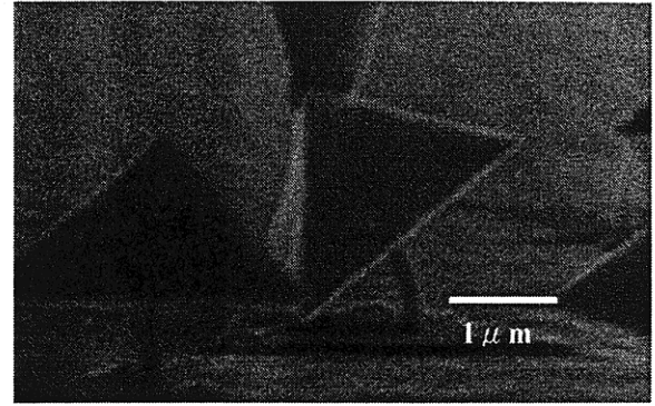
Figure 8: SEM image of a bonded SOI based oscillator being bent with a straight neck. The neck is seen to bend equally among the length.
