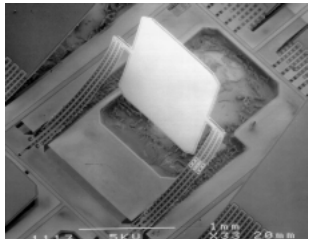
Fig. 6: SEM picture of a free-standing, mobile, flat plate of density modulated porous silicon lifted out of plane by two actuator arms. The plate contains 256 double layers with high and low indices of refraction. Dimensions: 1100\text{ }\mu\text{m} \times 1850\text{ }\mu\text{m} \times 30\text{ }\mu\text{m} .
