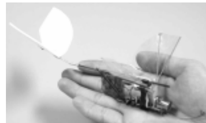
Figure 14: Battery-powered ornithopter MAV
