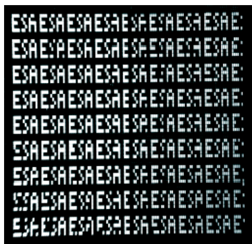
Figure 9. A 2-D addressing pattern from a flight-format 365x171 microshutter array showing “ESA” letters
