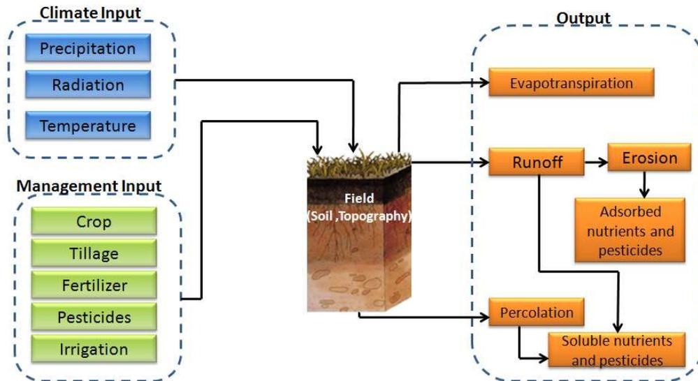
Figure 1. GLEAMS model schema (modified from Thomas, 2009)
