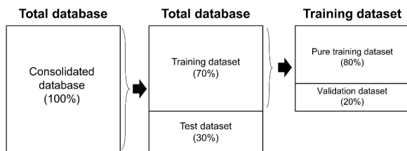
Fig. 11. Schematic diagram for dataset preparation by random selection for machine learning algorithm implementation.
