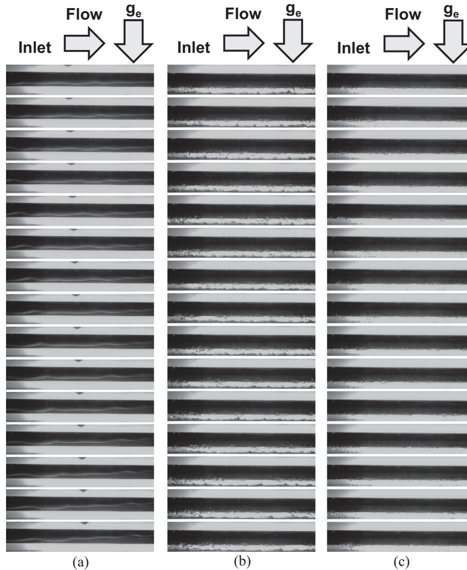
Fig. 3. Sequential images of horizontal flow captured at the middle of the channel ( z = 294 mm) with (a) G_{FC} = 17.9 kg/m 2 s, G_{H_2O} = 462.8 kg/m 2 s, P_{FC,in} = 124.0 kPa, P_{WT_{BH}} = 315.3 , and x_{e,in} = 1.06 , (b) G_{FC} = 67.3 kg/m 2 s, G_{H_2O} = 462.0 kg/m 2 s, P_{FC,in} = 125.5 kPa, P_{WT_{BH}} = 1108.8 , and x_{e,in} = 1.12 , and (c) G_{FC} = 99.6 kg/m 2 s, G_{H_2O} = 462.1 kg/m 2 s, P_{FC,in} = 125.2 kPa, P_{WT_{BH}} = 1575.2 , and x_{e,in} = 1.12 , with individual images in each sequence separated by 0.01 s.
