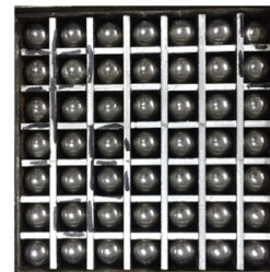
(e) Grille-particle channel with \delta_g=2.6 mm and d_p=12 mm (G1P3)
