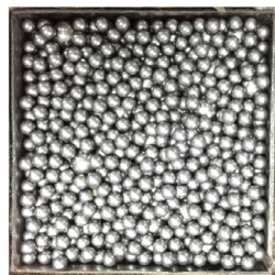
(a) Particle channel with d_p=6 mm (P1)
