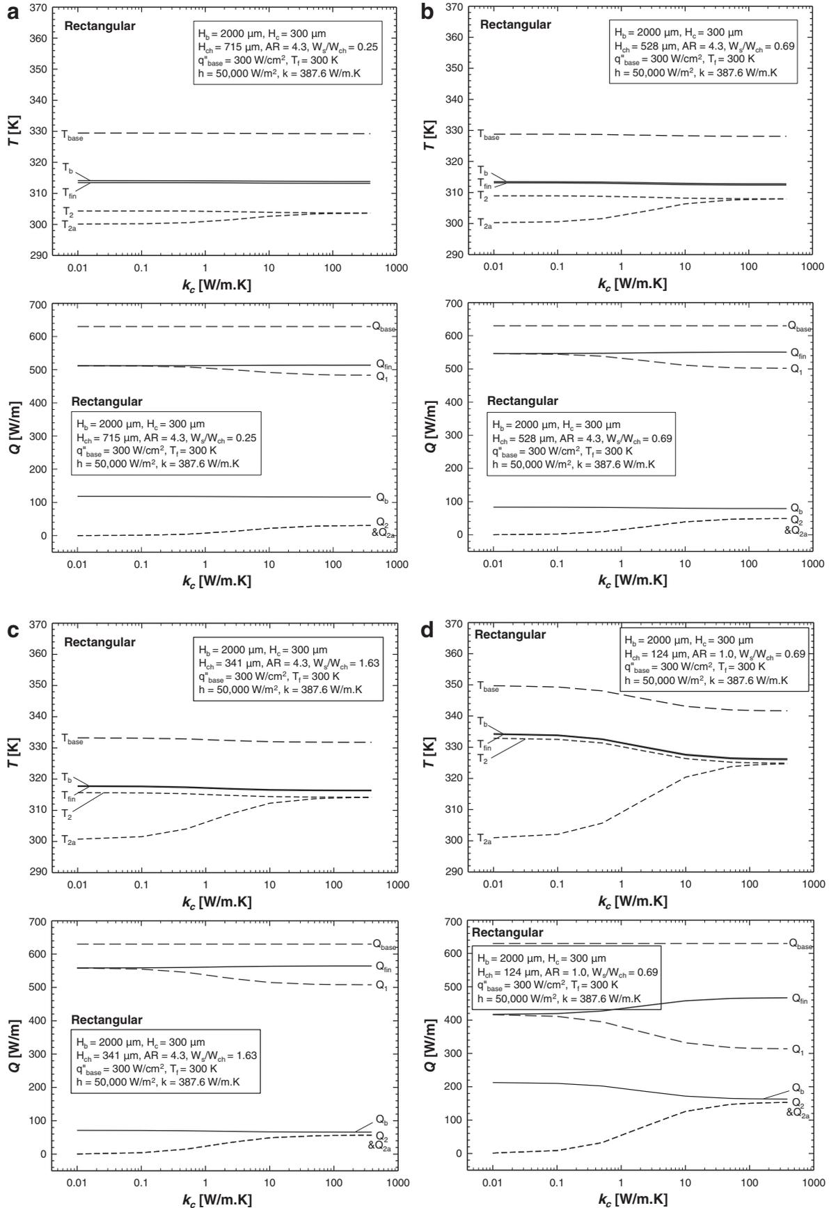
Fig. 5. Effects of thermal conductivity of cover plate for rectangular channel with (a)  $H_{ch} = 715 \mu\text{m}$ , (b)  $H_{ch} = 528 \mu\text{m}$ , (c)  $H_{ch} = 341 \mu\text{m}$  and (d)  $H_{ch} = 124 \mu\text{m}$ .
