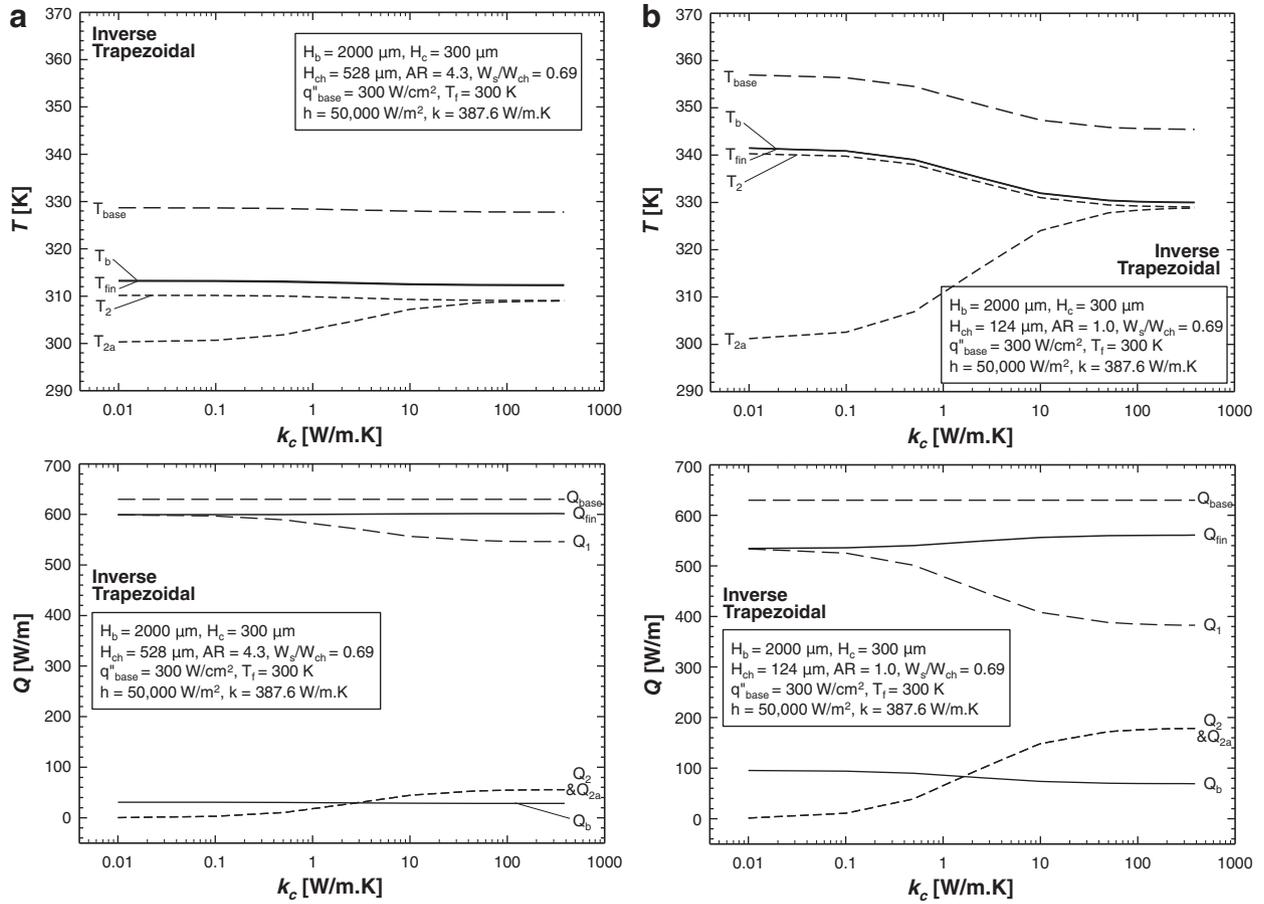
Fig. 6. Effects of thermal conductivity of cover plate for inverse trapezoidal channel with (a)  $H_{ch} = 528 \mu\text{m}$  and (b)  $H_{ch} = 124 \mu\text{m}$ .
