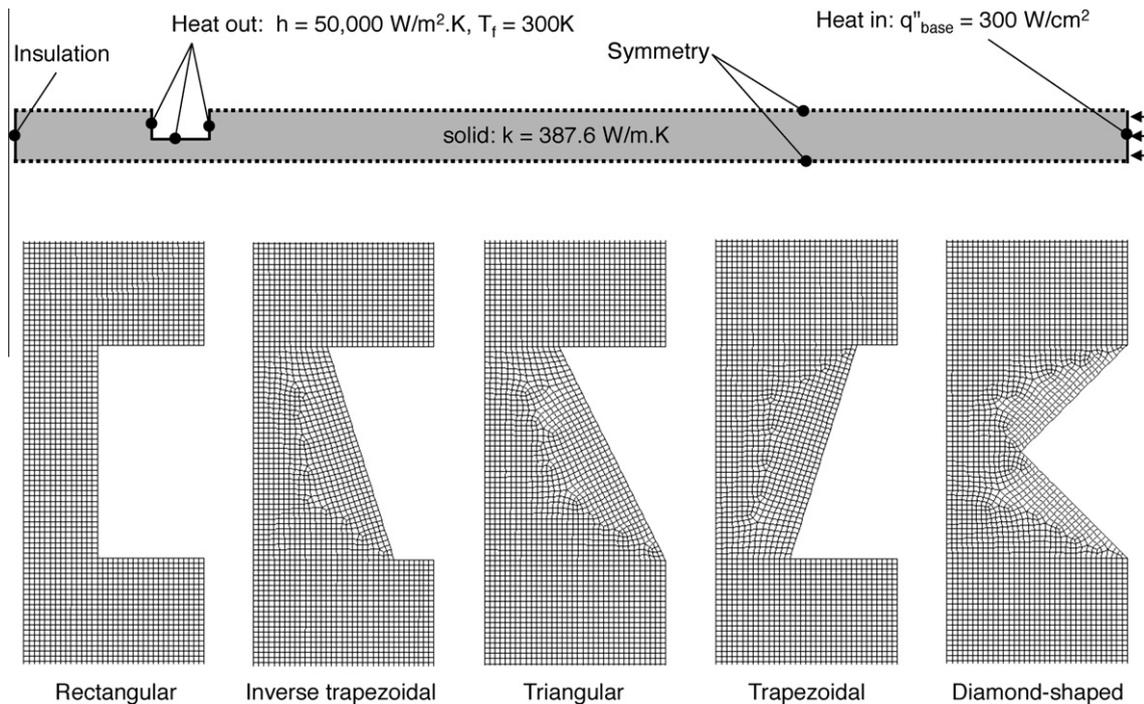
**Fig. 4.** Sample computational domain (shown turned 90°) of monolithic heat sink with rectangular cross-section and  $H_{ch} = 124 \mu\text{m}$ , with magnification of micro-channel cross-sections for all five cross-sections with same channel height.
