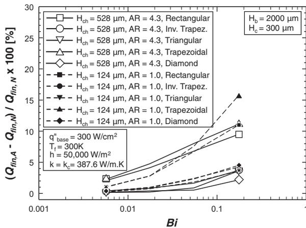
Fig. 9. Variation of percent difference between analytical and two-dimensional numerical results with Biot number for  $W_s/W_{ch} = 0.69$ .
