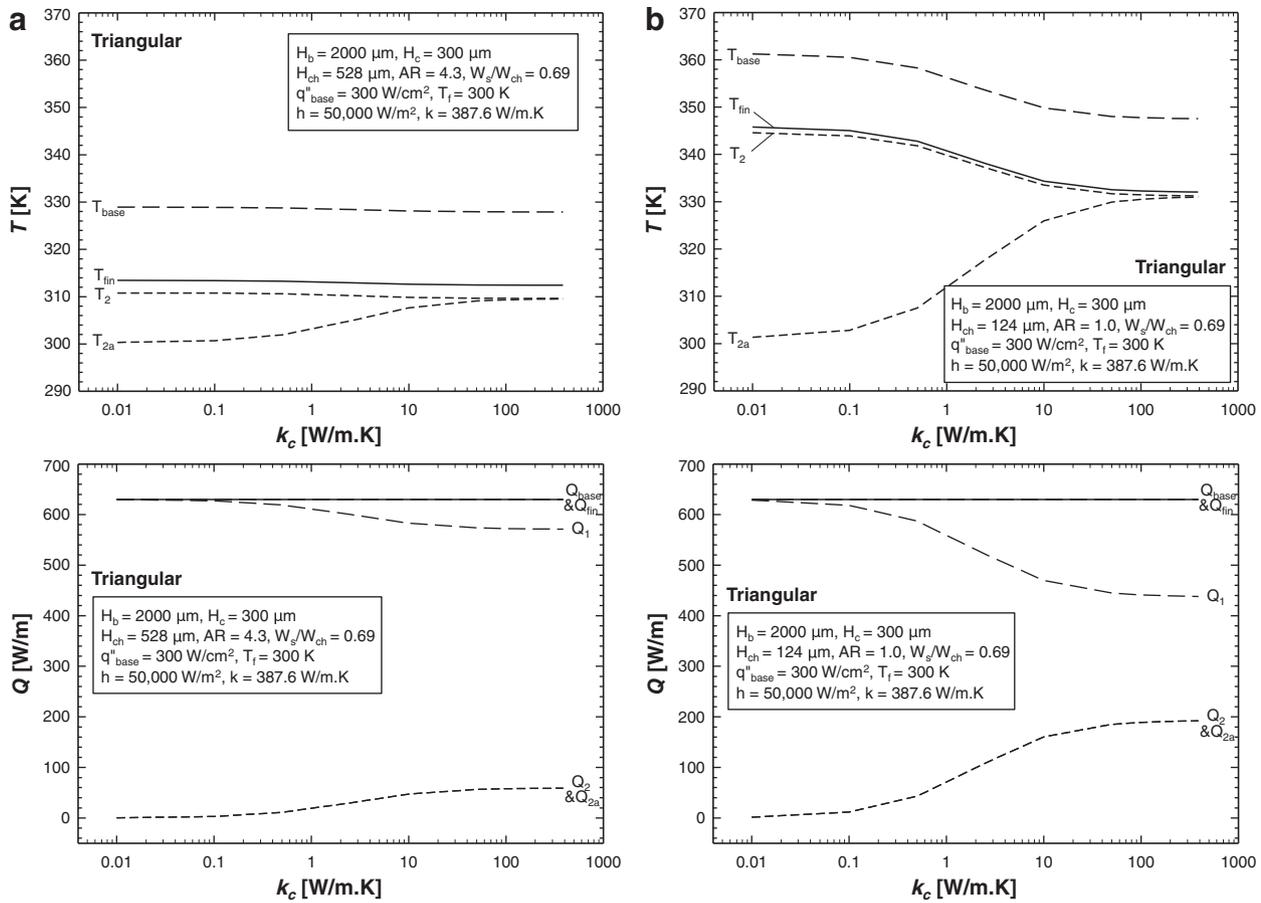
Fig. 7. Effects of thermal conductivity of cover plate for triangular channel with (a)  $H_{ch} = 528 \mu\text{m}$  and (b)  $H_{ch} = 124 \mu\text{m}$ .
