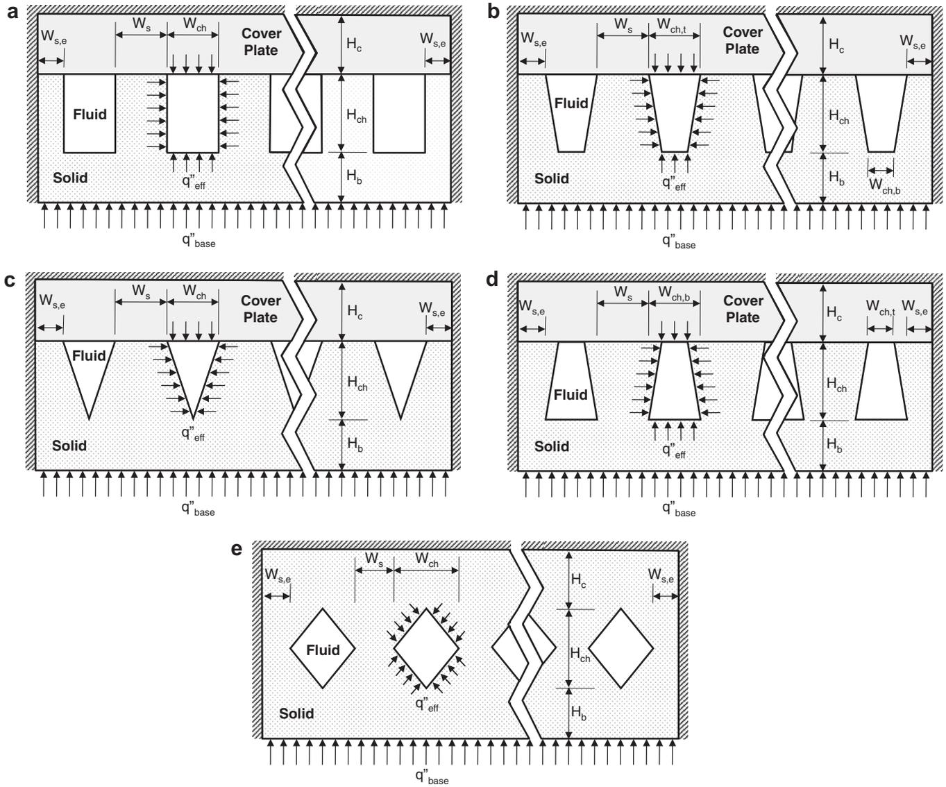
Fig. 1. Schematic diagrams of micro-channel heat sinks with (a) rectangular, (b) inverse-trapezoidal, (c) triangular, (d) trapezoidal, and (e) diamond-shaped cross-sections.
