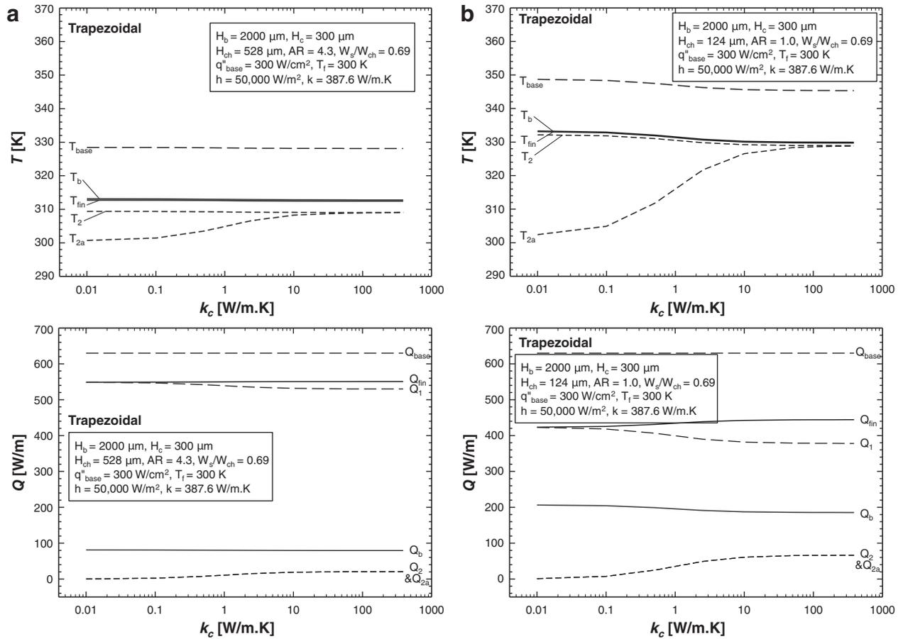
Fig. 8. Effects of thermal conductivity of cover plate for trapezoidal channel with (a)  $H_{ch} = 528 \mu\text{m}$  and (b)  $H_{ch} = 124 \mu\text{m}$ .
