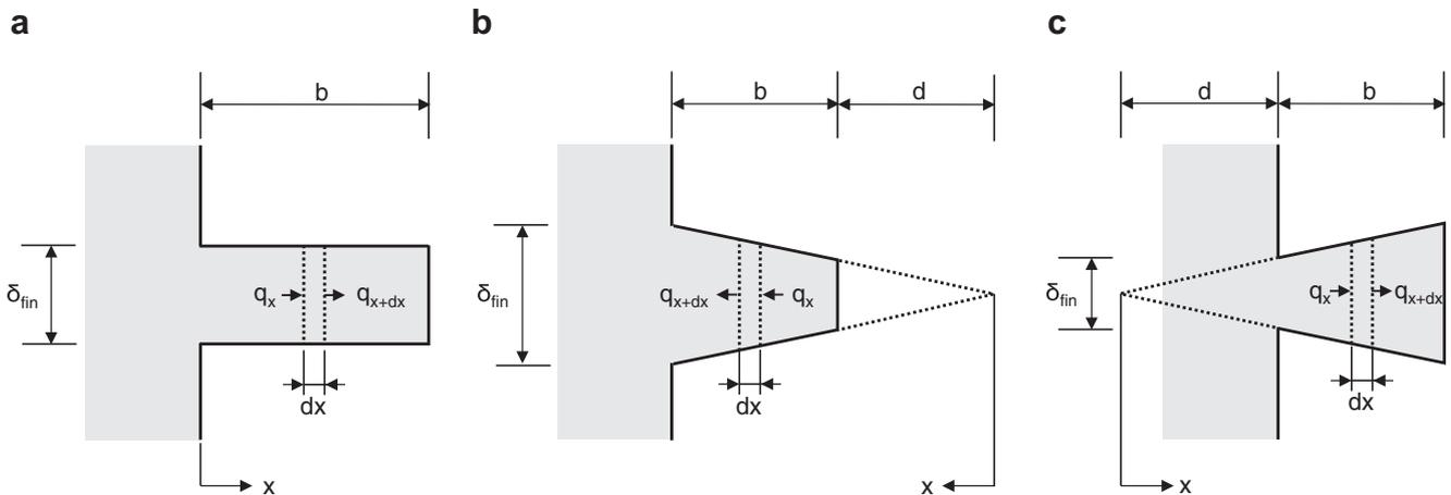
Fig. 2. Schematic diagrams of (a) rectangular, (b) trapezoidal and (c) inverse trapezoidal fins.
