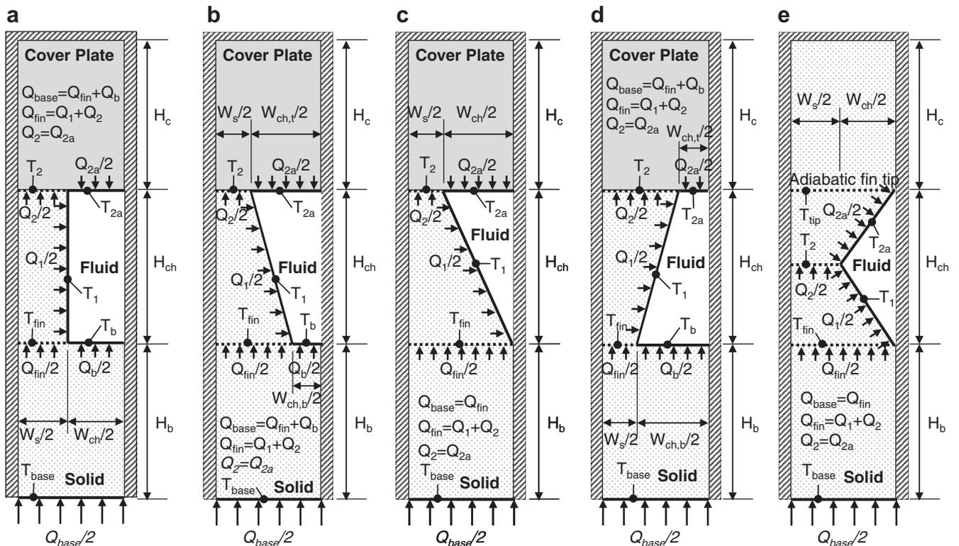
Fig. 3. Heat sink unit cells with: (a) rectangular, (b) inverse trapezoidal, (c) triangular, (d) trapezoidal, and (e) diamond-shaped micro-channel cross-sections.
