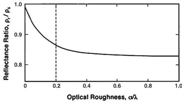
Fig. 2. Ratio of normal hemispherical reflectance versus optical roughness for aluminum coated ground glass (adapted from [8]).
