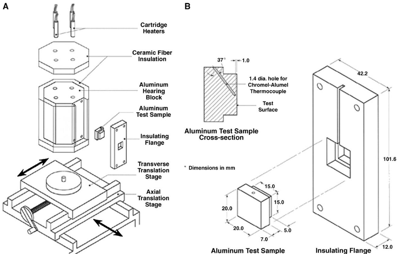
Fig. 1. Construction of (a) sample heating assembly and (b) test sample and insulating flange.
