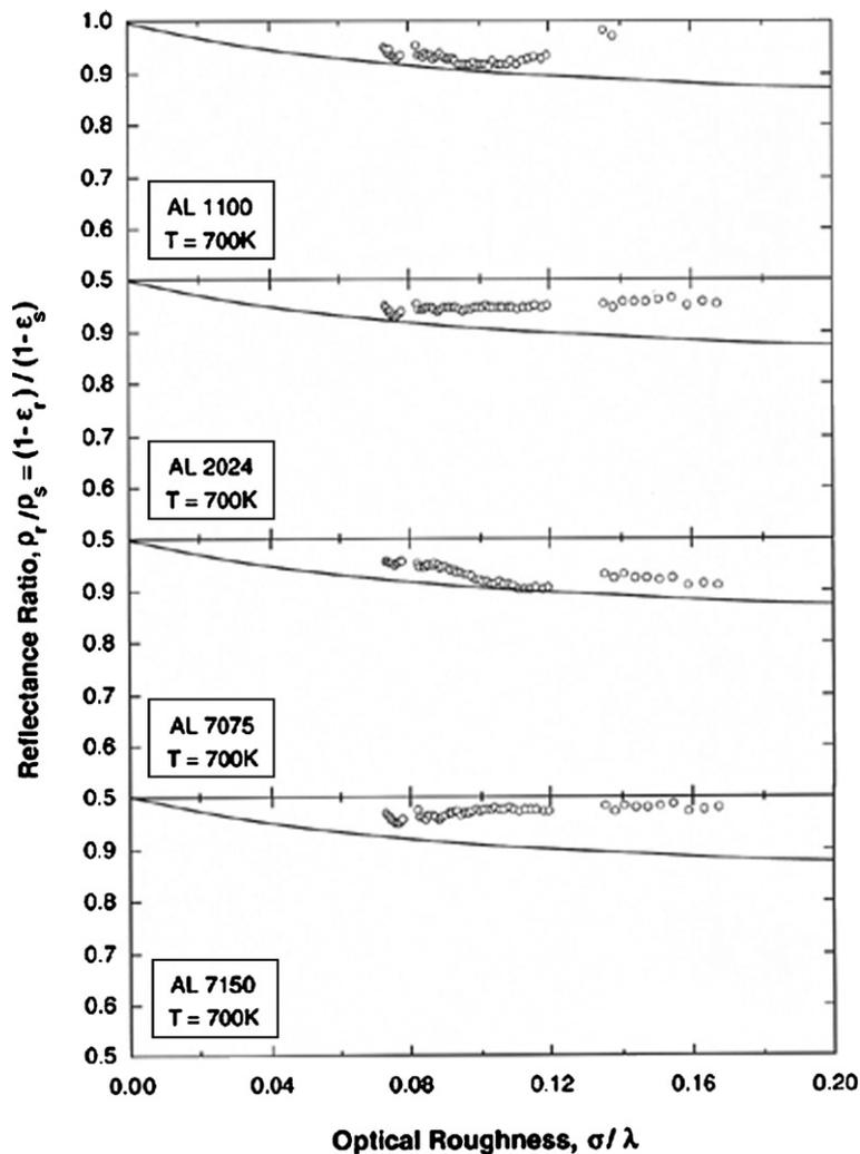
Fig. 4. Present normal hemispherical reflectance values versus optical roughness for different alloys at 700 K compared with Eq. (9).
