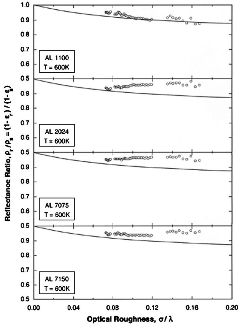
Fig. 3. Present normal hemispherical reflectance values versus optical roughness for different alloys at 600 K compared with Eq. (9).
