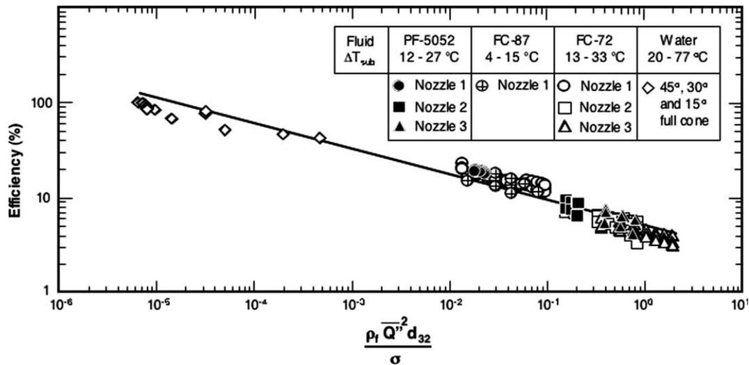
Fig. 10. Evaporation efficiency versus Weber number. PF-5052 data are for upward-oriented sprays, FC-87, FC-72 and water downward-oriented.
