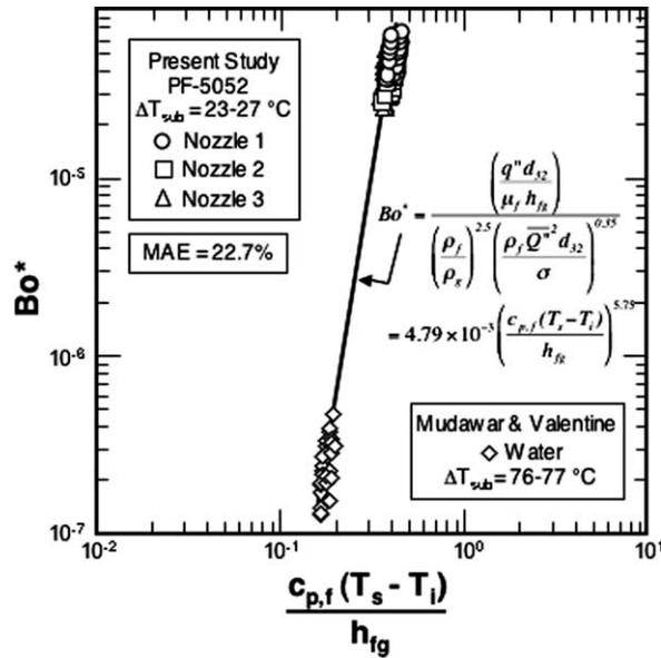
Fig. 8. Nucleate boiling correlation for upward-oriented PF-5052 sprays and downward-oriented water sprays.
