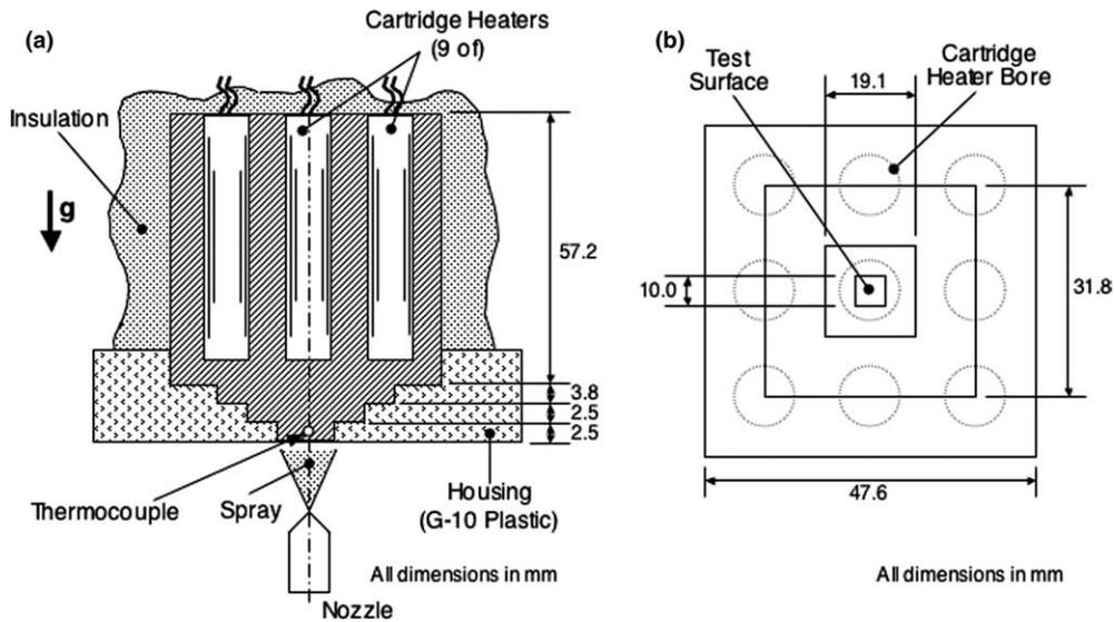
Fig. 3. (a) Longitudinal section of heater assembly and (b) bottom view of copper block.
