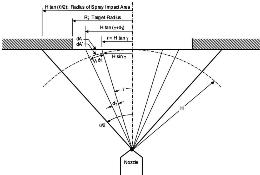
Fig. 4. Spray volumetric flux distribution for uniform point source (adapted from Mudawar and Estes [11]).
