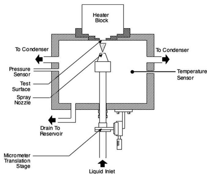
Fig. 2. Schematic of spray chamber.
