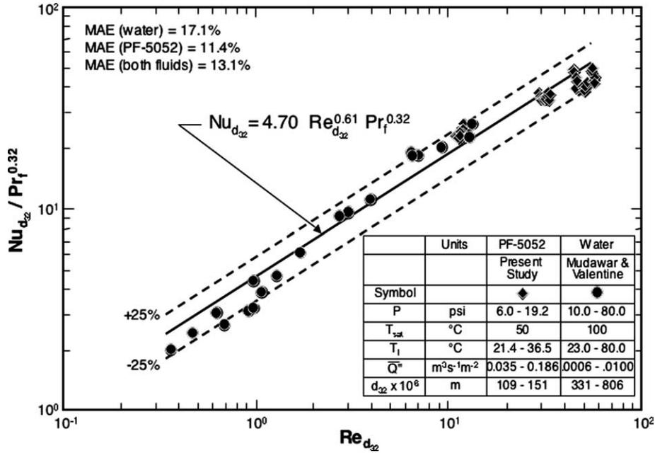
Fig. 7. Single-phase heat transfer correlation for upward-oriented PF-5052 sprays and downward-oriented water sprays.
