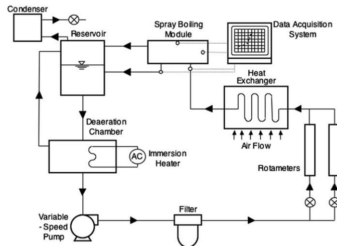
Fig. 1. Two-phase spray cooling flow loop.
