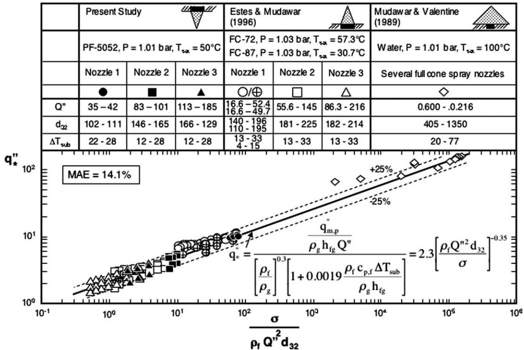
Fig. 9. Correlation of CHF data for all fluids, orientations and nozzles based on volumetric flux at outer circumference of impact area.
