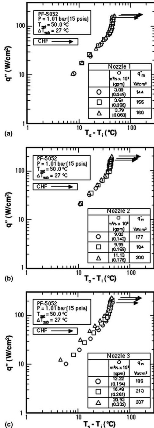
Fig. 5. Boiling curves for different flow rates at  $\Delta T_{sub} = 27^\circ\text{C}$  for (a) nozzle 1, (b) nozzle 2, and (c) nozzle 3.
