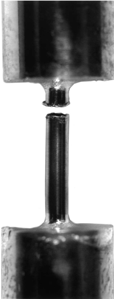
Fig. 4. AISI type 304 stainless steel test section ( D = 0.902 mm, t_w = 0.089 mm, L/D = 6.4 ) following burnout.
