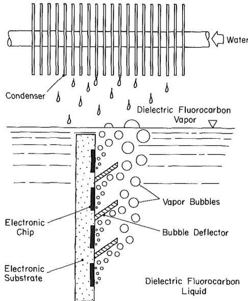
Fig. 1 Schematic representation of the encapsulated pool boiling thermosyphon cooling system
