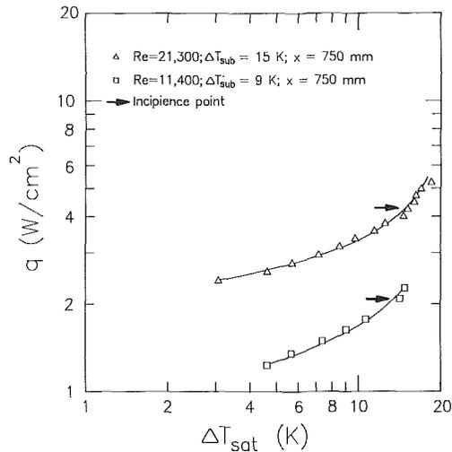
Fig. 9 Boiling curves corresponding to position  $x = 750$  mm
