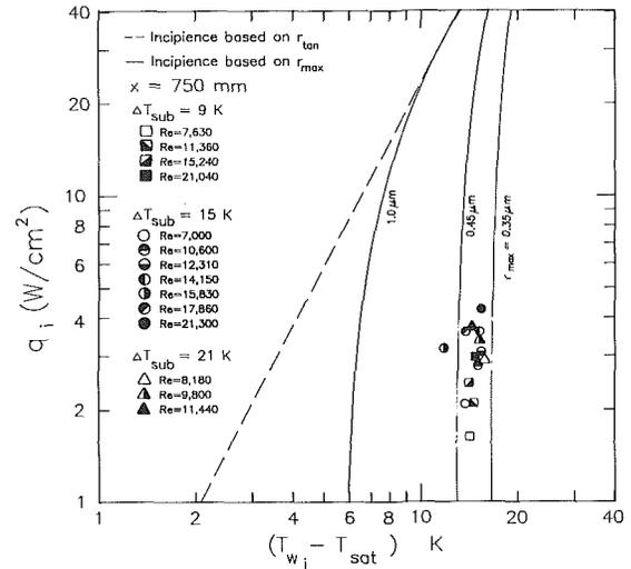
Fig. 11 Incipience conditions at position  $x = 750$  mm
