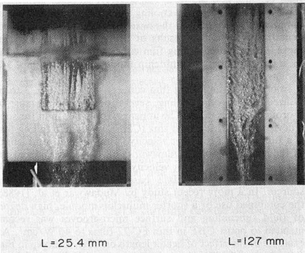
Fig. 4 Photographs of CHF in a falling film on a vertical rectangular heated surface at  $U = 0.5$  m/s and  $L = 25.4$  and  $127$  mm, respectively
