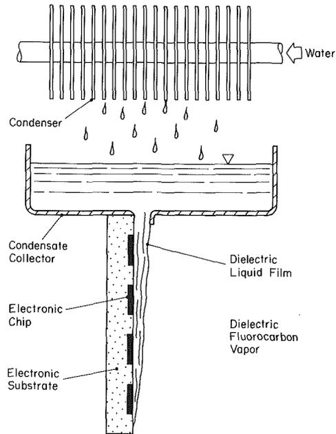
Fig. 2 Schematic representation of a passive falling-film thermosyphon cooling system
