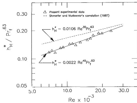
Fig. 8 Correlation of the dimensionless heat transfer coefficient
