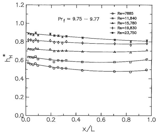
Fig. 7 Variation of the dimensionless heat transfer coefficient along the heated length for  $Pr_f = 9.75-9.77$
