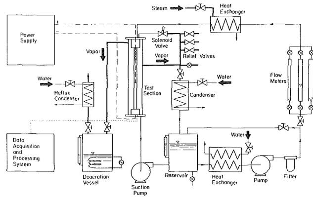
Fig. 5 Schematic diagram of the fluid delivery system
