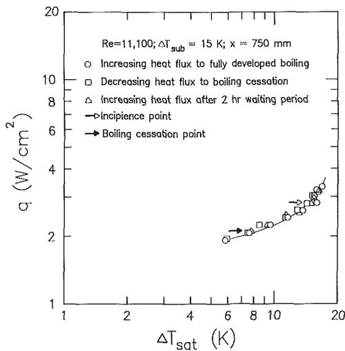
Fig. 10 Boiling curves corresponding to position  $x = 750$  mm
