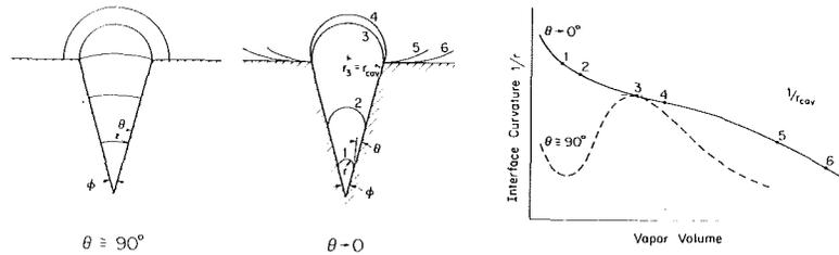
Fig. 13 Schematic representation of vapor embryo growth for highly wetting fluids
