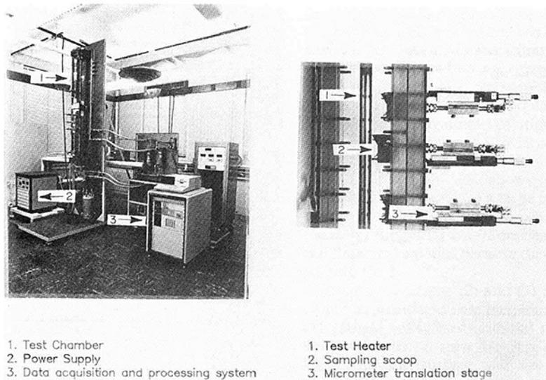
Fig. 6 Photographs of the test facility and sampling scoops
