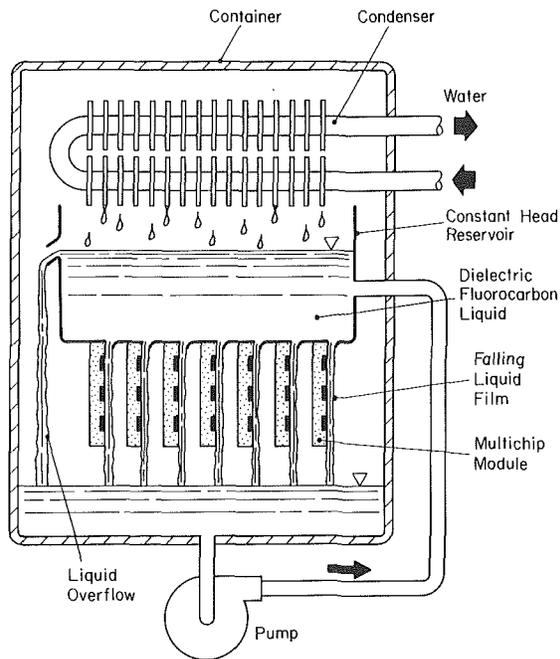
Fig. 3 Schematic of the semi-passive falling-film electronic cooling system
