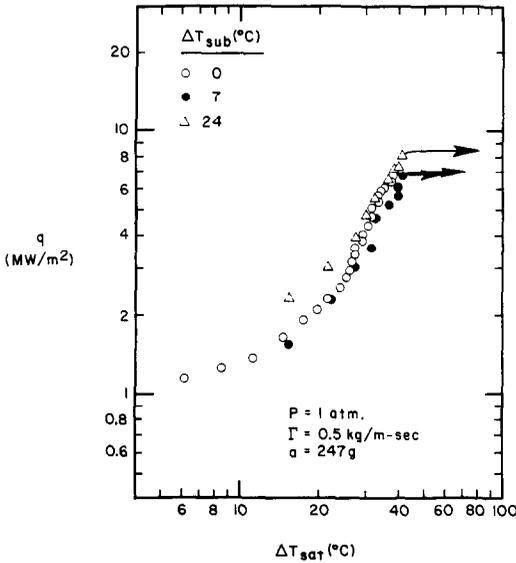
FIG. 5. Effect of subcooling on heat transfer.
