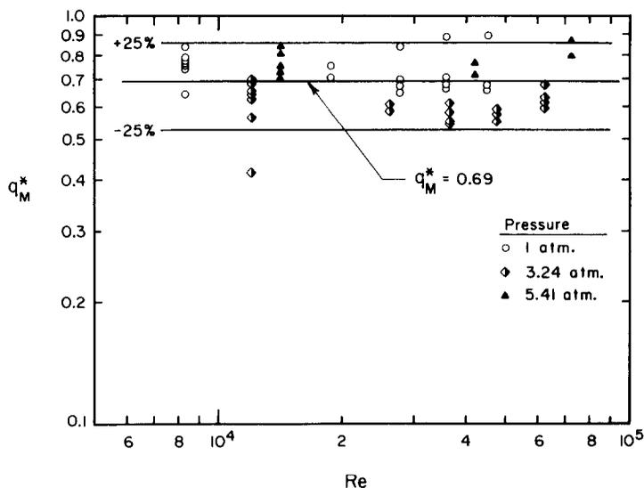
FIG. 16. CHF correlation based on the Coriolis-force model.
