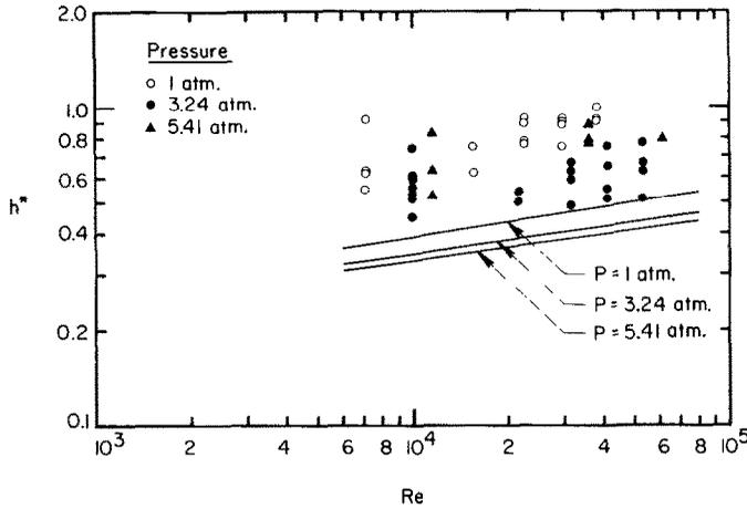
FIG. 9. Comparison of experimental and calculated heat transfer coefficient.
