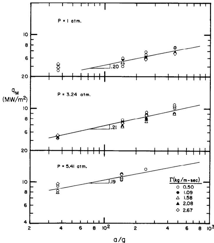
FIG. 15. Effect of centrifugal acceleration on CHF.
