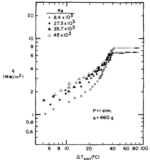
FIG. 8. Effect of flow rate on heat transfer.
