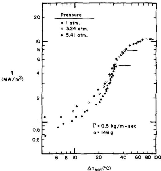
FIG. 6. Effect of pressure on heat transfer.
