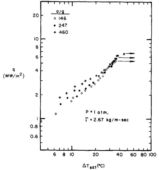
FIG. 7. Effect of rotation on heat transfer.
