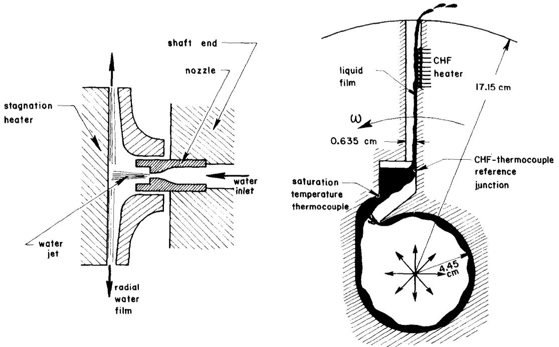
FIG. 2. Impingement jet flow against the surface of the stagnation heater and the spiral film flow inside the rotating disc.
