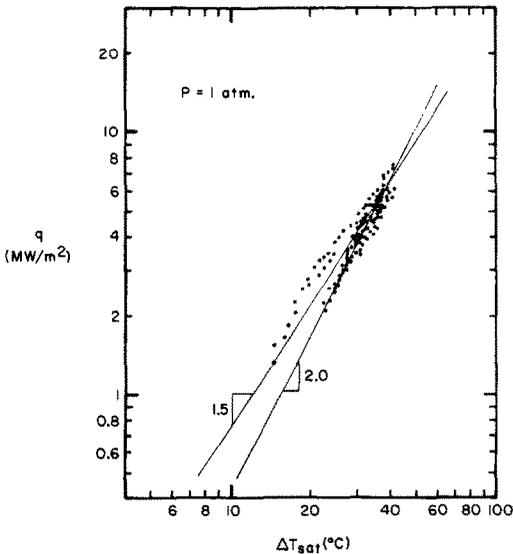
FIG. 10. Fully-developed boiling data at 1 atm.
