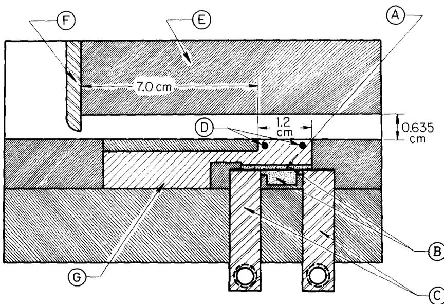
FIG. 3. Construction of the CHF probe. A: ribbon heater; B: boron nitride plates; C: stainless steel electric power terminals; D: thermocouples; E: G-7 plastic insulator (used in most of the probe pieces); F: nozzle plate; G: copper block.
