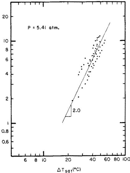
FIG. 12. Fully-developed boiling data at 5.41 atm.
