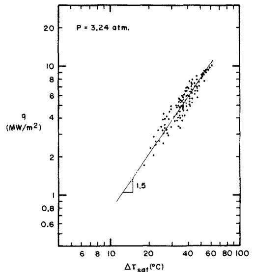
FIG. 11. Fully-developed boiling data at 3.24 atm.
