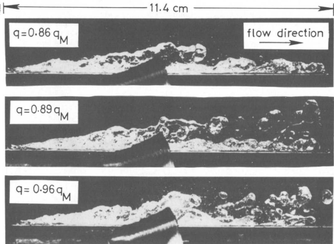
FIG. 13. Successive stages of film breakdown leading to CHF in inclined-plane water films obtained by Baines [8] ( $u_0 = 0.83 \text{ m s}^{-1}$ ,  $q_M = 1.252 \text{ MW m}^{-2}$ ). The object shown in the middle of each figure is external and did not interfere with the flow.
