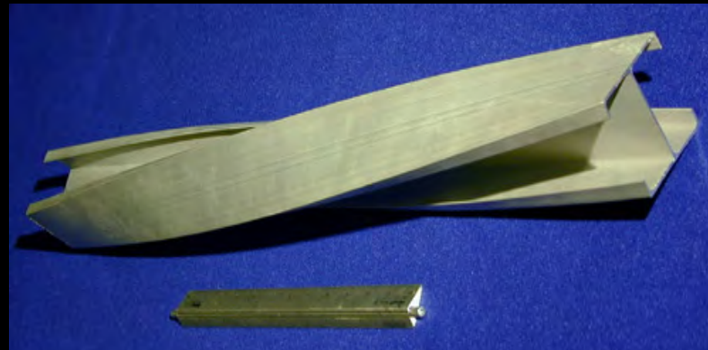
Distortion induced by Poor Quenching
