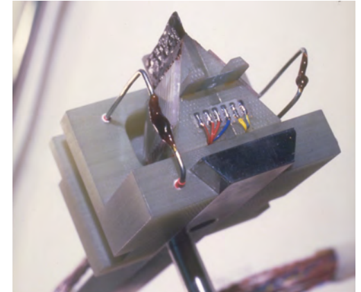
Thermocouple Knife-edge for Measurement of Temperature Profile across Wavy Liquid Layer
