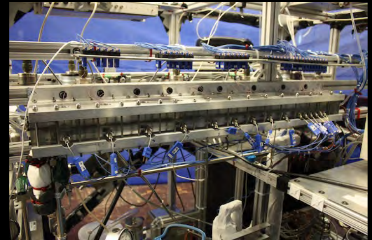
CM-HT: Condensation Module for Heat Transfer Measurements
