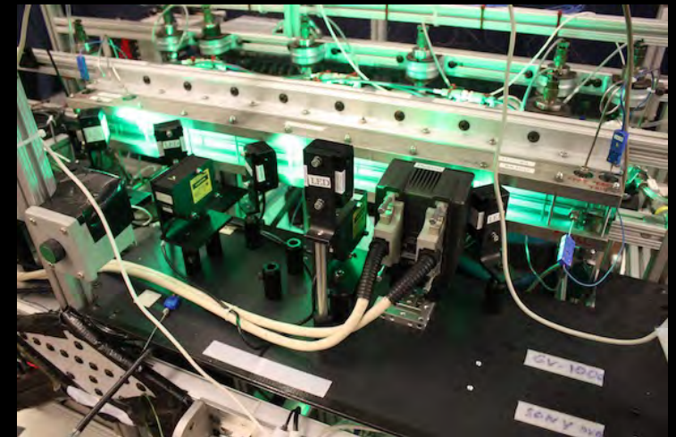
CM-FV: Condensation Module for Flow Visualization
