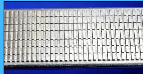
Cross-flow Micro-channel Heat Exchanger Facility for Study of Air-fuel Heat Transfer in High Mach Turbine Engines
