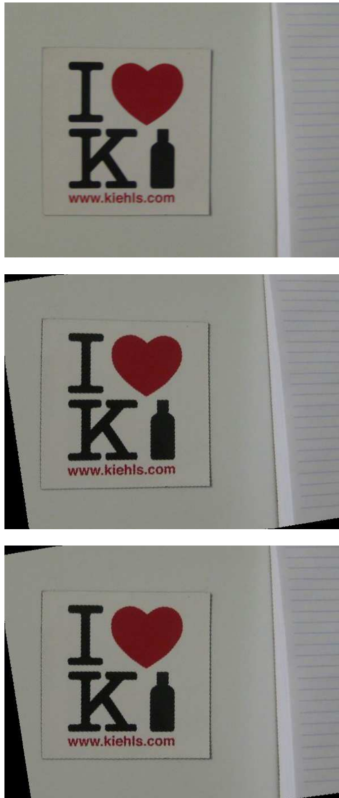
Figure 10: Up: original image m1a.jpg; middle: transformed m1b.jpg (mse:85.71) by best H obtained by 4 corner point pairs; down: transformed m1b.jpg (mse:55.78) by H calculated from all inliers (44 in all)
