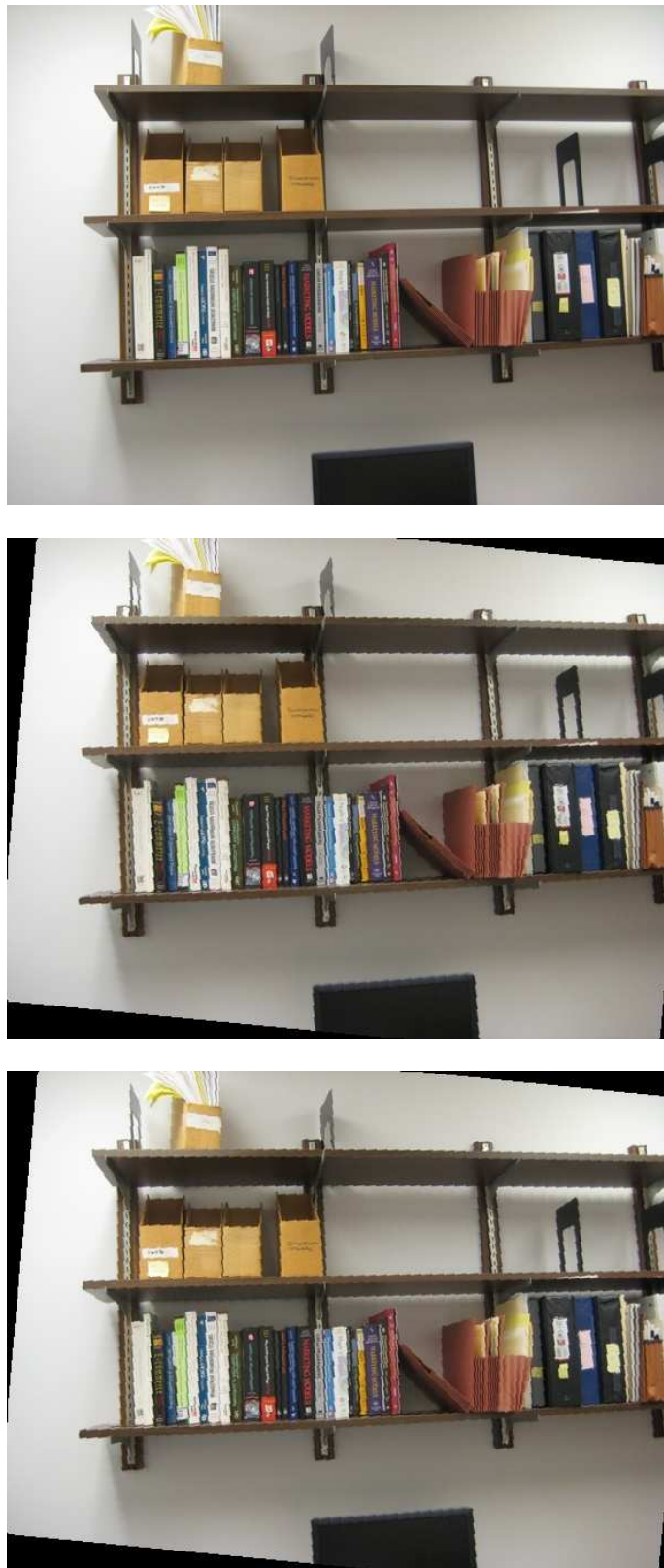
Figure 15: Up: original image m2a.jpg; middle: transformed m2b.jpg (mse:184.07) by best H obtained by 4 corner point pairs; down: transformed m2b.jpg (mse:150.35) by H calculated from all inliers (39 in all)
