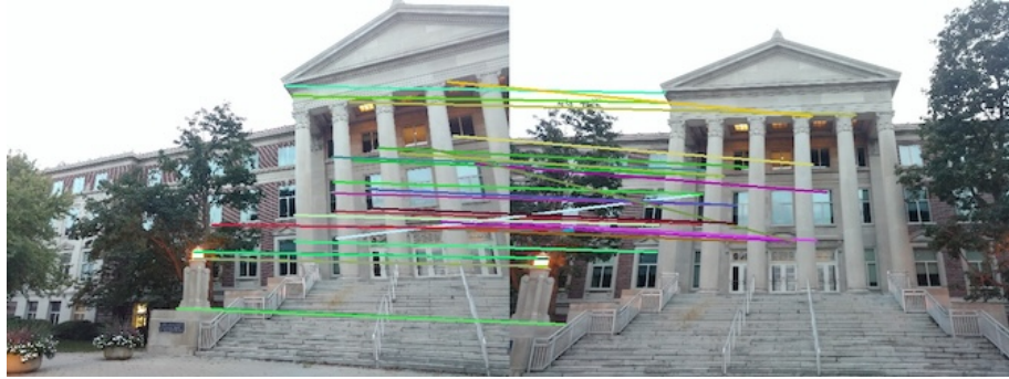
Figure 12: Matching in image pair 1 (using NCC and \sigma = 1.2 )
