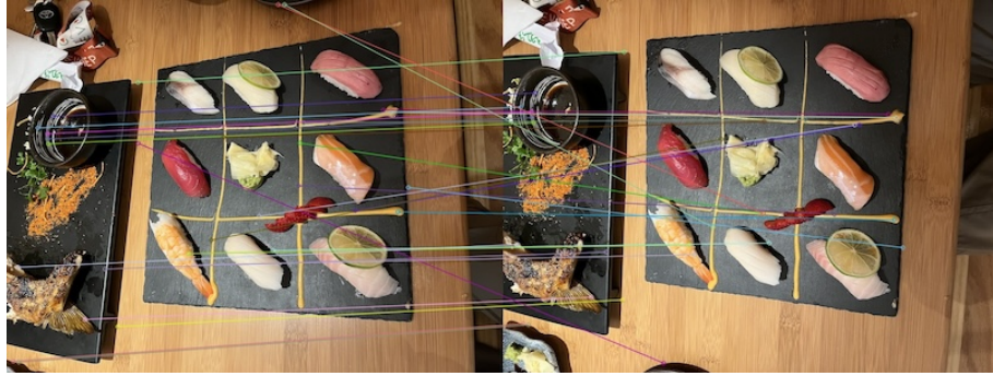
Figure 57: Matching in image pair 1 using SIFT
