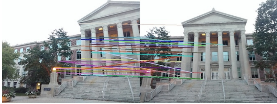
Figure 11: Matching in image pair 1 (using NCC and \sigma = 1 )
