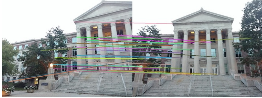
Figure 7: Matching in image pair 1 (using SSD and \sigma = 1 )
