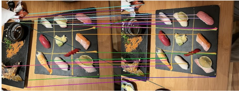
Figure 42: Matching in image pair 1 (using NCC and \sigma = 1.2 )
