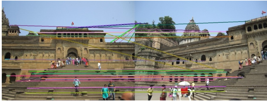
Figure 25: Matching in image pair 2 (using NCC and \sigma = 1.6 )
