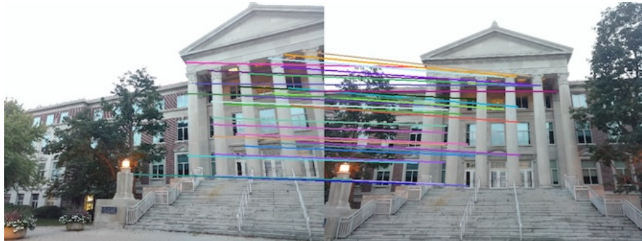
Figure 13: Matching in image pair 2 (using NCC and \sigma = 1.6 )
