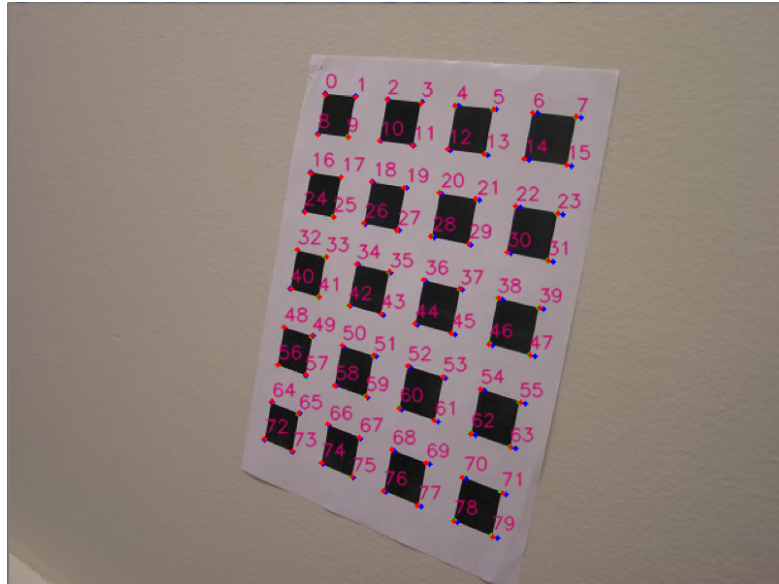
Figure 13: Dataset1 Sample 1: first example of re-projection results with labels. Green dots: ground truth extracted from Canny and Hough lines. Blue dots: re-projection on the image plane using the initial camera parameter. Red dots: re-projection on the image plane using the LM-optimized camera parameter.
