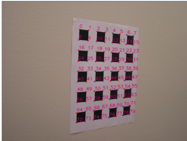
Figure 14: Dataset1 Sample 2: second example of re-projection results with labels. Green dots: ground truth extracted from Canny and Hough lines. Blue dots: re-projection on the image plane using the initial camera parameter. Red dots: re-projection on the image plane using the LM-optimized camera parameter.
