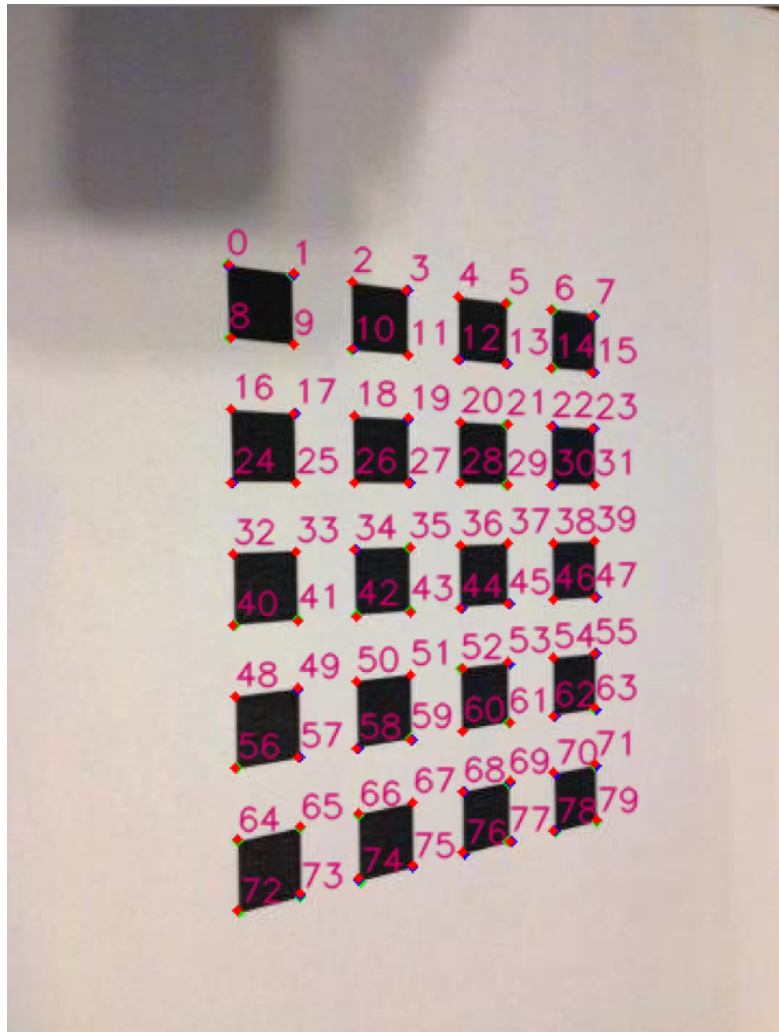
Figure 32: Dataset 2 Sample 4: fourth example of re-projection results with labels. Green dots: ground truth extracted from Canny and Hough lines. Blue dots: re-projection on the image plane using the initial camera parameter. Red dots: re-projection on the image plane using the LM-optimized camera parameter.
