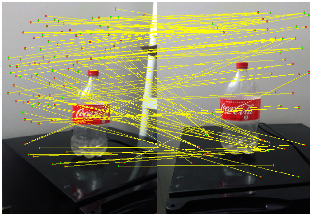
Figure 30: SSD on the Harris Corners on image pair 4 with \sigma = 1 .
