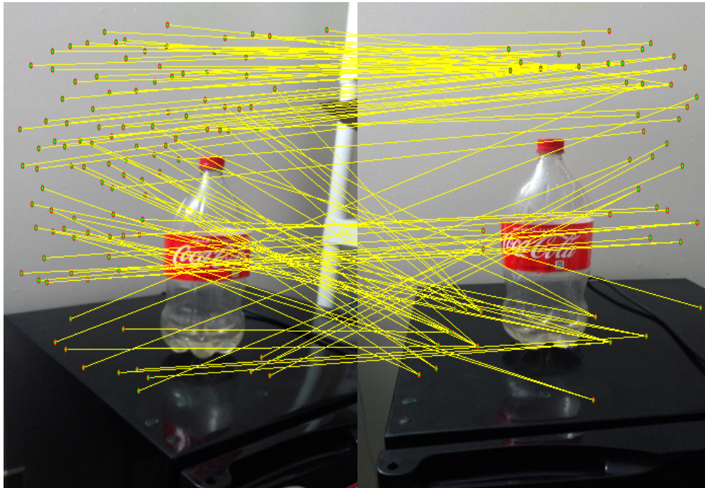
Figure 29: SSD on the Harris Corners on image pair 4 with \sigma = 0.707 .
