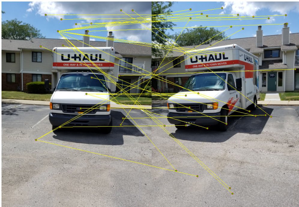
Figure 15: SSD on the Harris Corners on image pair 2 with \sigma = 1.414 .
