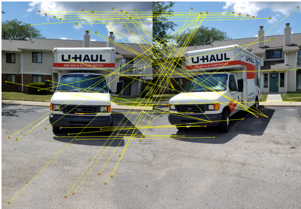
Figure 13: SSD on the Harris Corners on image pair 2 with \sigma = 0.707 .
