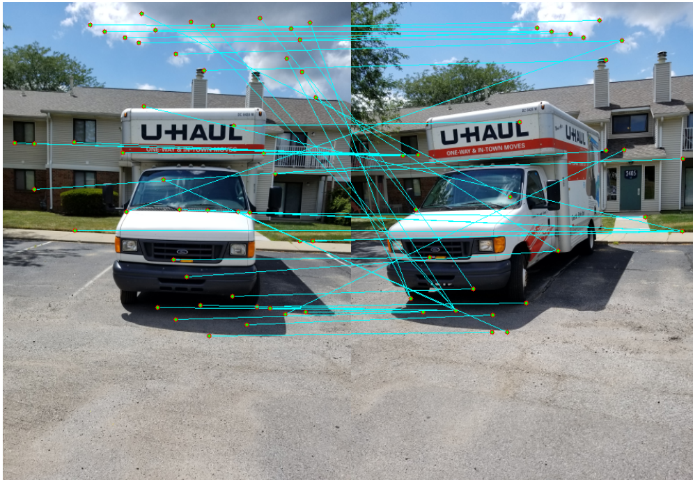
Figure 17: NCC on the Harris Corners on image pair 2 with \sigma = 0.707 .
