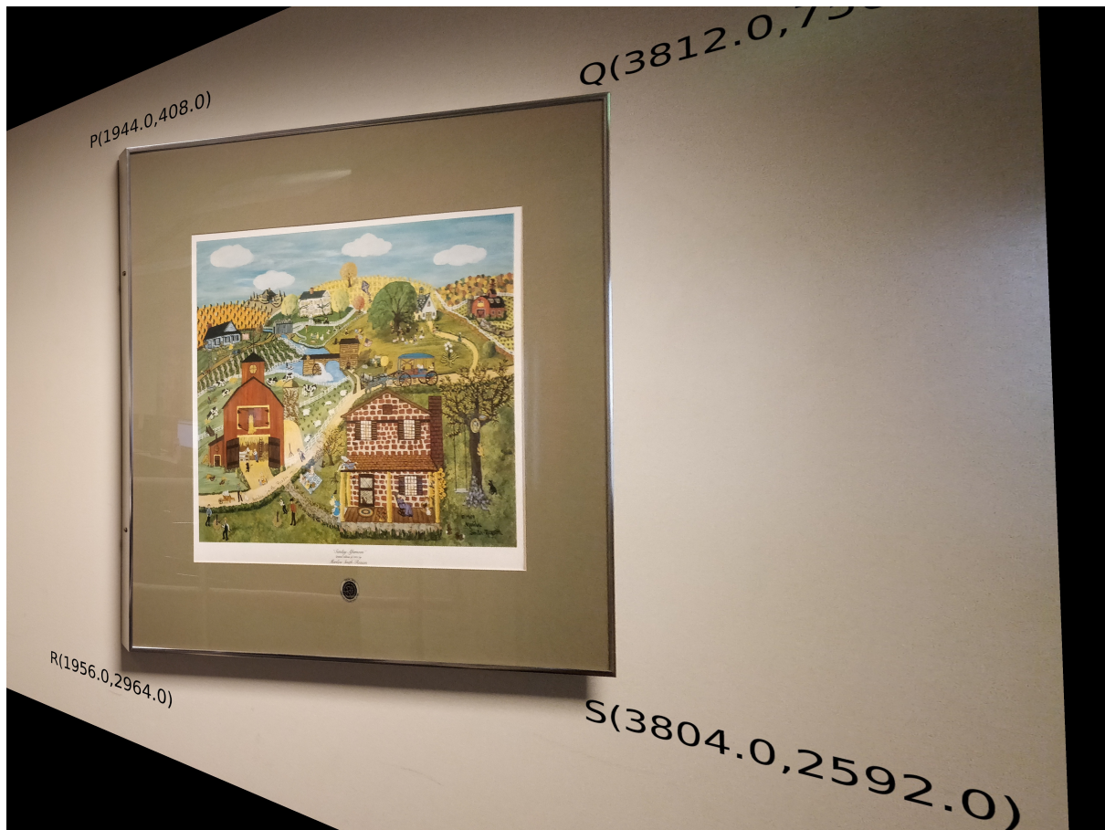
Figure 16: The resultant image when the product homography H_{ac} is applied to first frame plane with coordinates P, Q, R and S for Task 2
