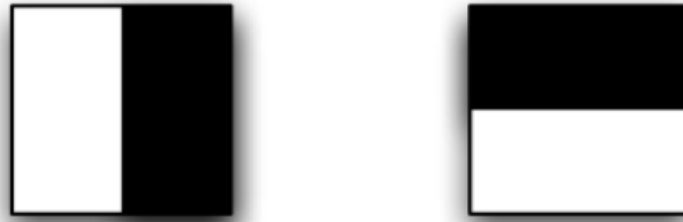
Figure 2: HAAR like feature detectors used to extract features from the image. The white part indicates the 0 region and the black part indicates the 1 region
