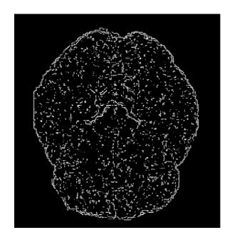
In this case, we can improve our result by smoothing the image with Gaussian low-pass filter of  $\sigma$  = 2.5 , then apply the Otsu's method.
