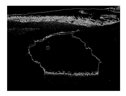
In this case, we can improve our result by smoothing the image with Gaussian low-pass filter of  $\sigma$  = 2.5 , then apply the Otsu's method.
