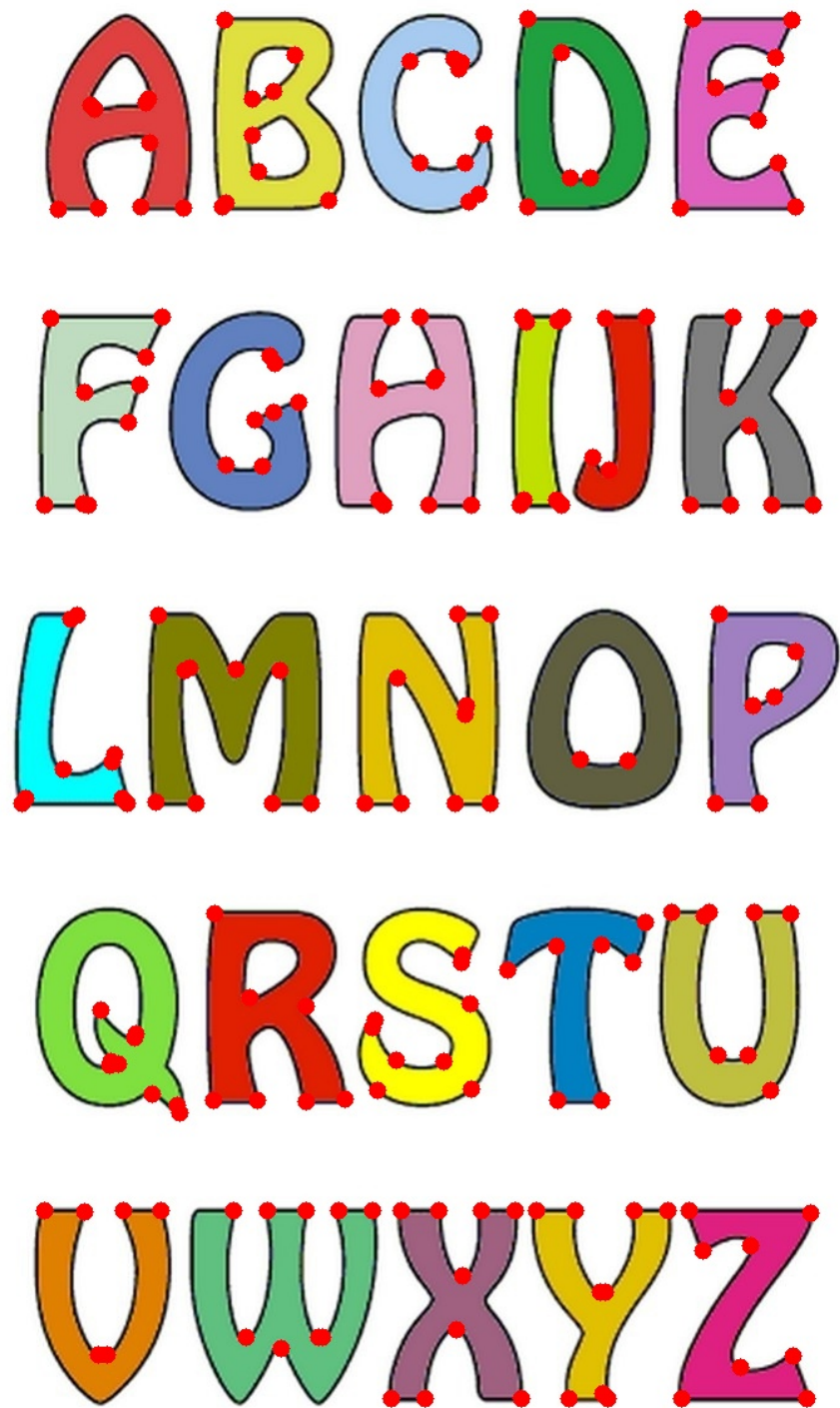
Figure 15: Harris corners (red circles) for each component. Note that some characters don't have enough corners. The number of corners per character will not exceed N = 9
