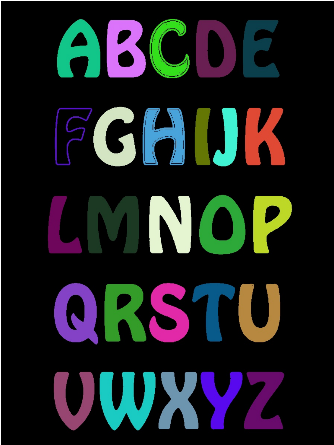
Figure 14: Component labeling: an image representing the output of the component labeling process. Each unique label (component) is given a random color for visualization. Note that this image is after the component cleaning process as well.
