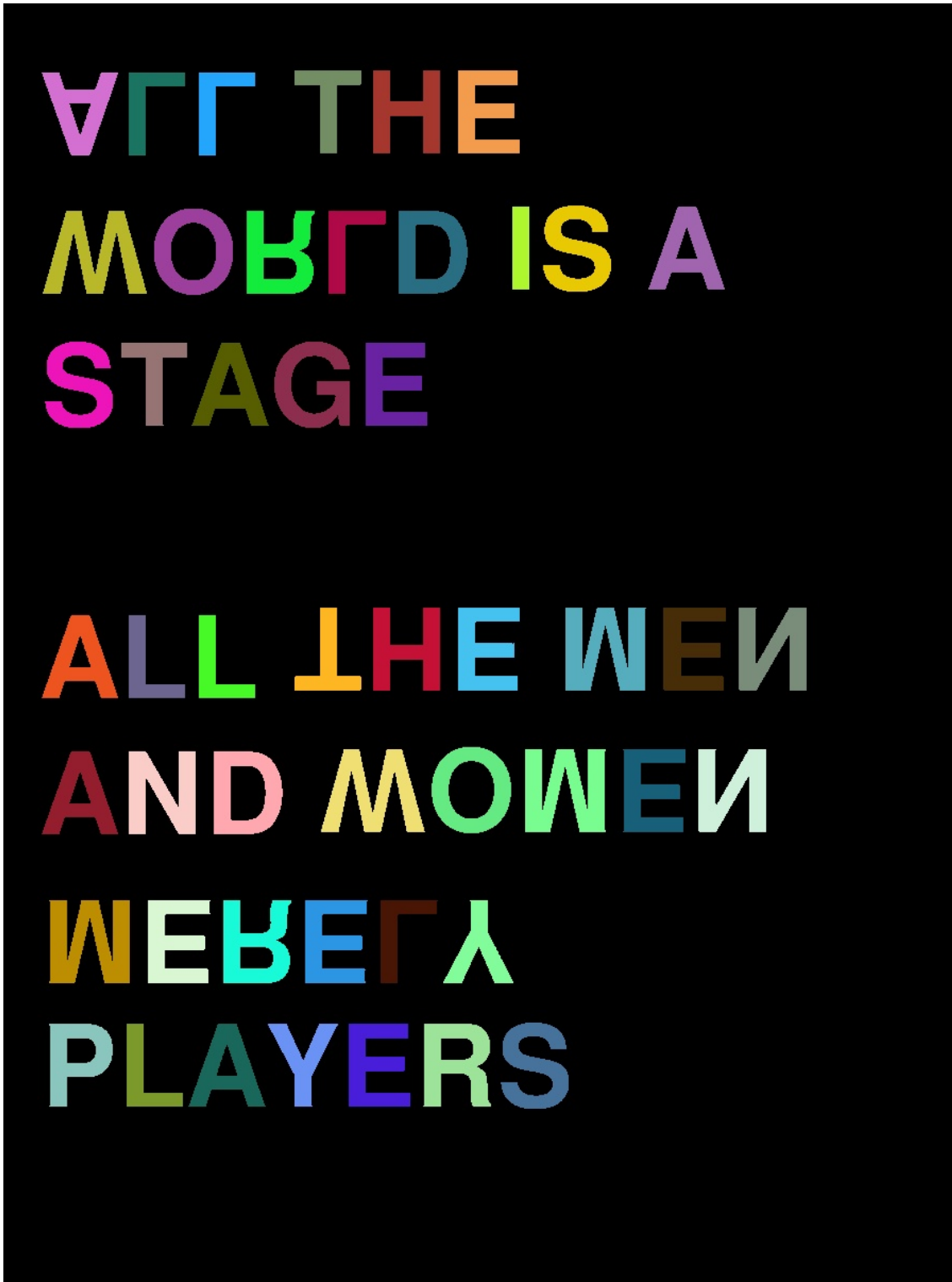
Figure 26: Component labeling: an image representing the output of the component labeling process. Each unique label (component) is given a random color for visualization. Note that this image is after the component cleaning process as well.
