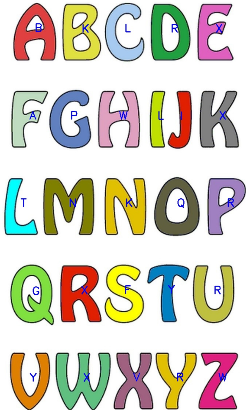
Figure 17: The output of the character recognition process. The overlaid blue characters are the output of the recognition process for the corresponding underlaid characters.
