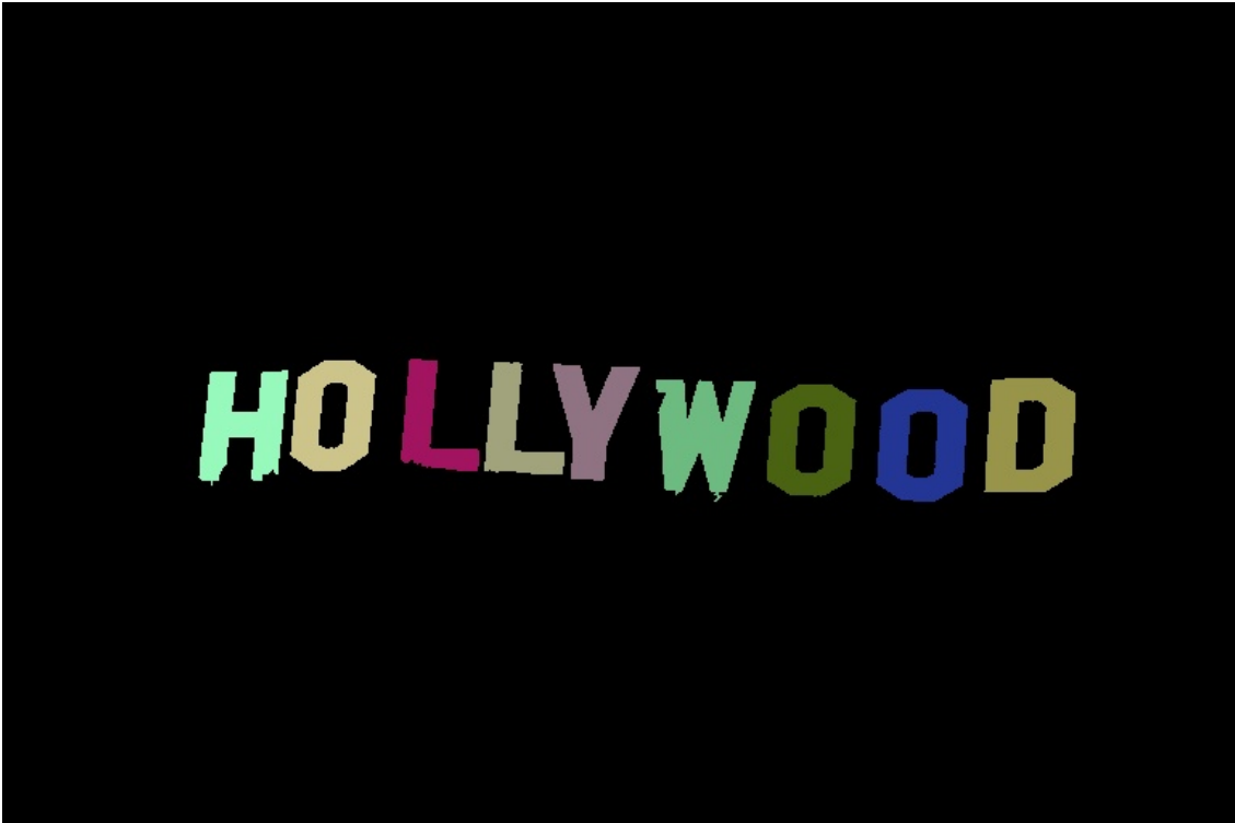
Figure 38: Component labeling: an image representing the output of the component labeling process. Each unique label (component) is given a random color for visualization. Note that this image is after the component cleaning process as well.
