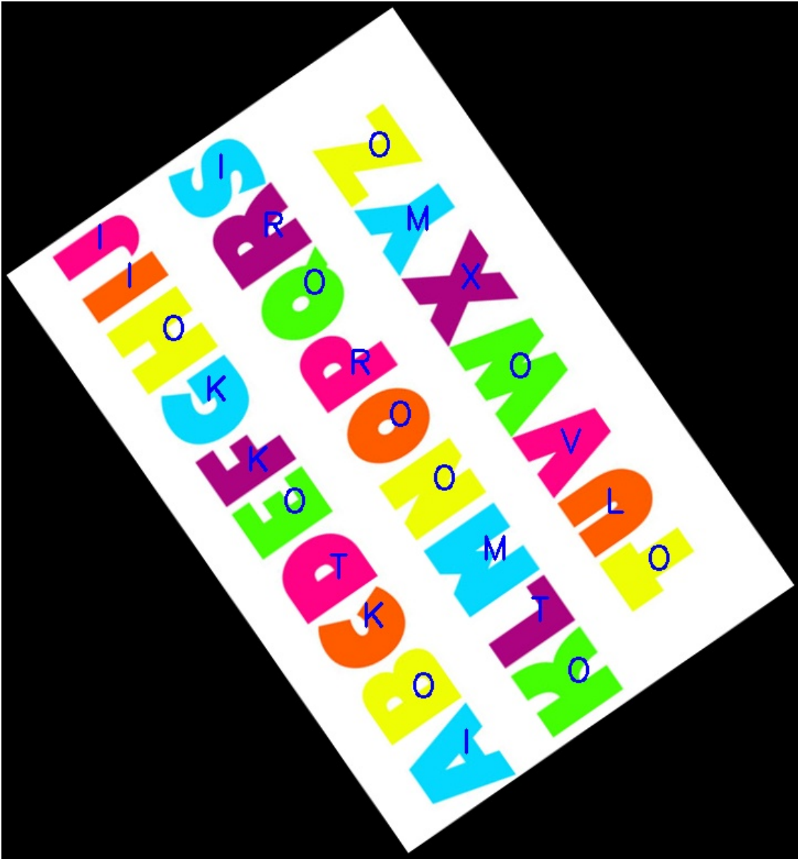
Figure 11: The output of the character recognition process. The overlaid blue characters are the output of the recognition process for the corresponding underlaid characters.
