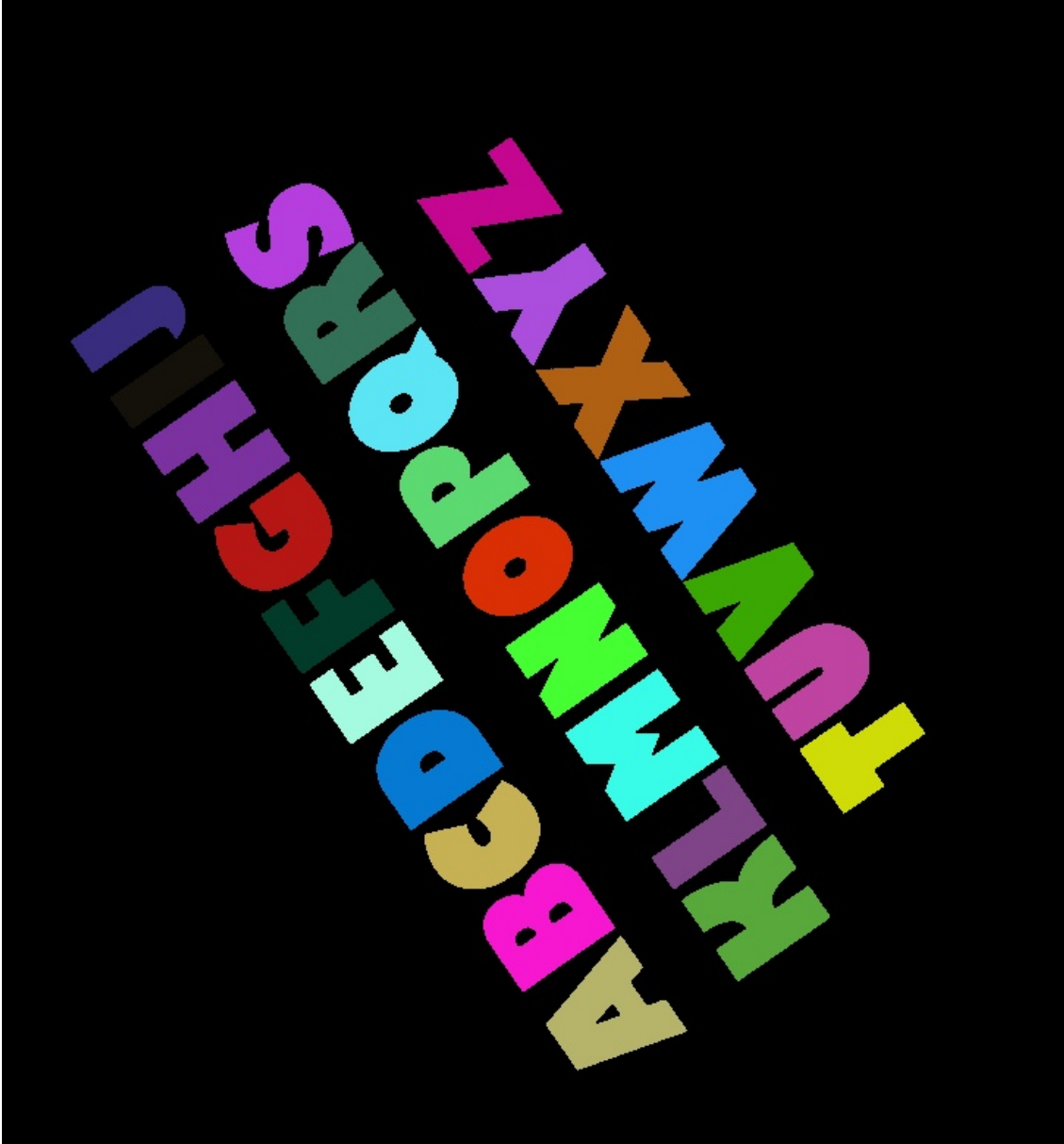
Figure 8: Component labeling: an image representing the output of the component labeling process. Each unique label (component) is given a random color for visualization. Note that this image is after the component cleaning process as well.
