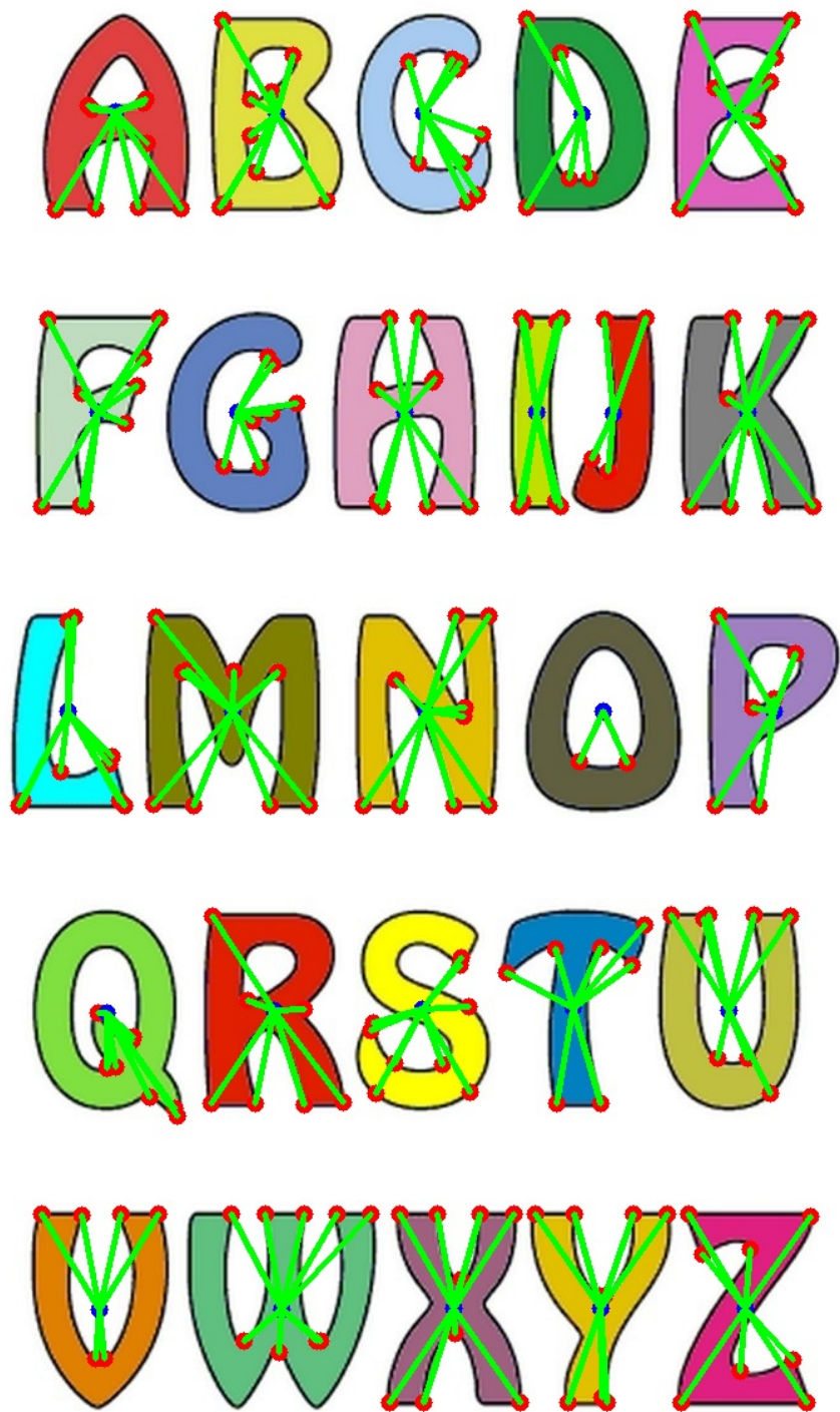
Figure 16: The shape vector of each component is the N-vector of angles between each successive pair of the N (green) lines that join the component center (blue) with the corners (red)
