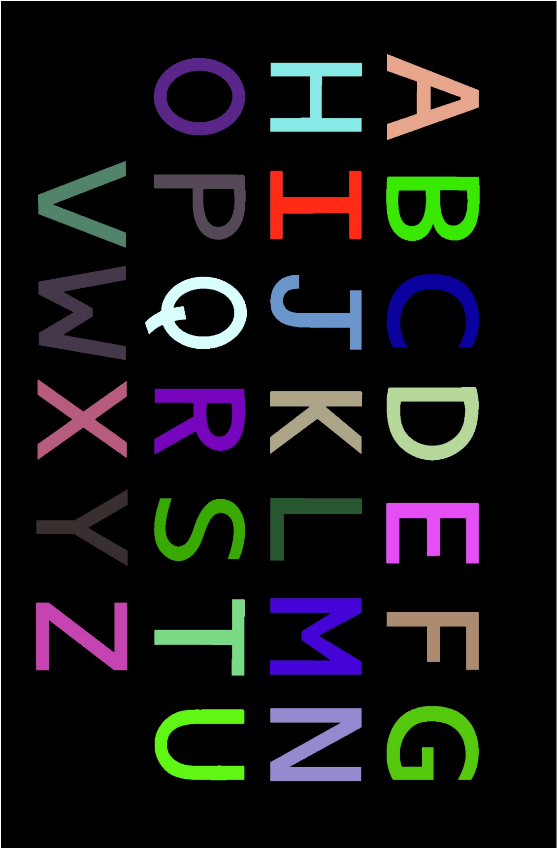
Figure 32: Component labeling: an image representing the output of the component labeling process. Each unique label (component) is given a random color for visualization. Note that this image is after the component cleaning process as well.
