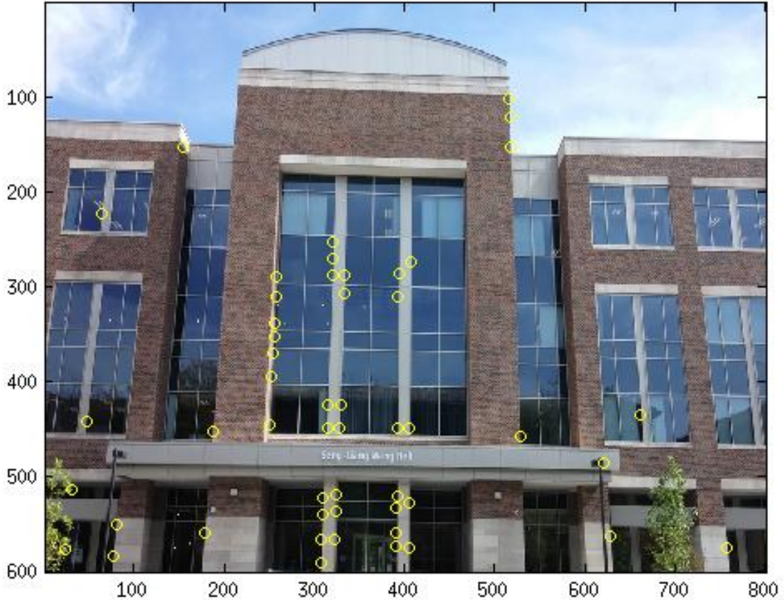
Fig 42. The corner points detected on pic2.jpg using \sigma = 1
