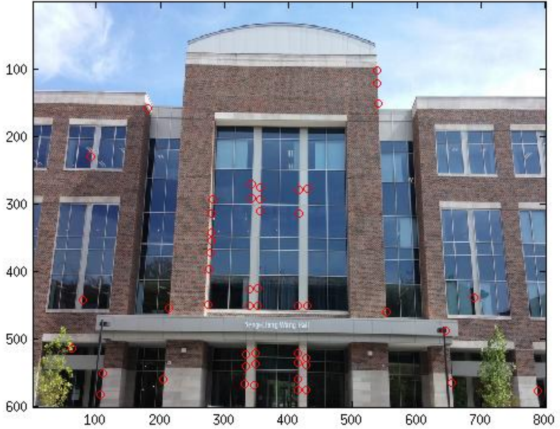
Fig 41. The corner points detected on pic1.jpg using \sigma = 1
