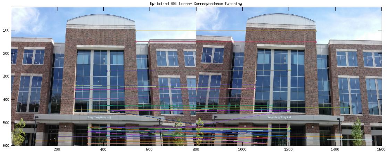
Figure 7. Harris: The SSD matching with \sigma = 1.4
