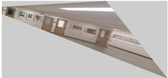
• Set 1: Img1.jpg – One-step Method: Projective and affine distortion removed
