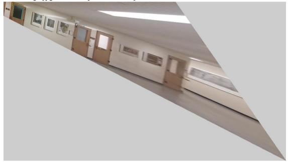
• *Set 1:* Img1.jpg – Two-step Method: Affine distortion removed
