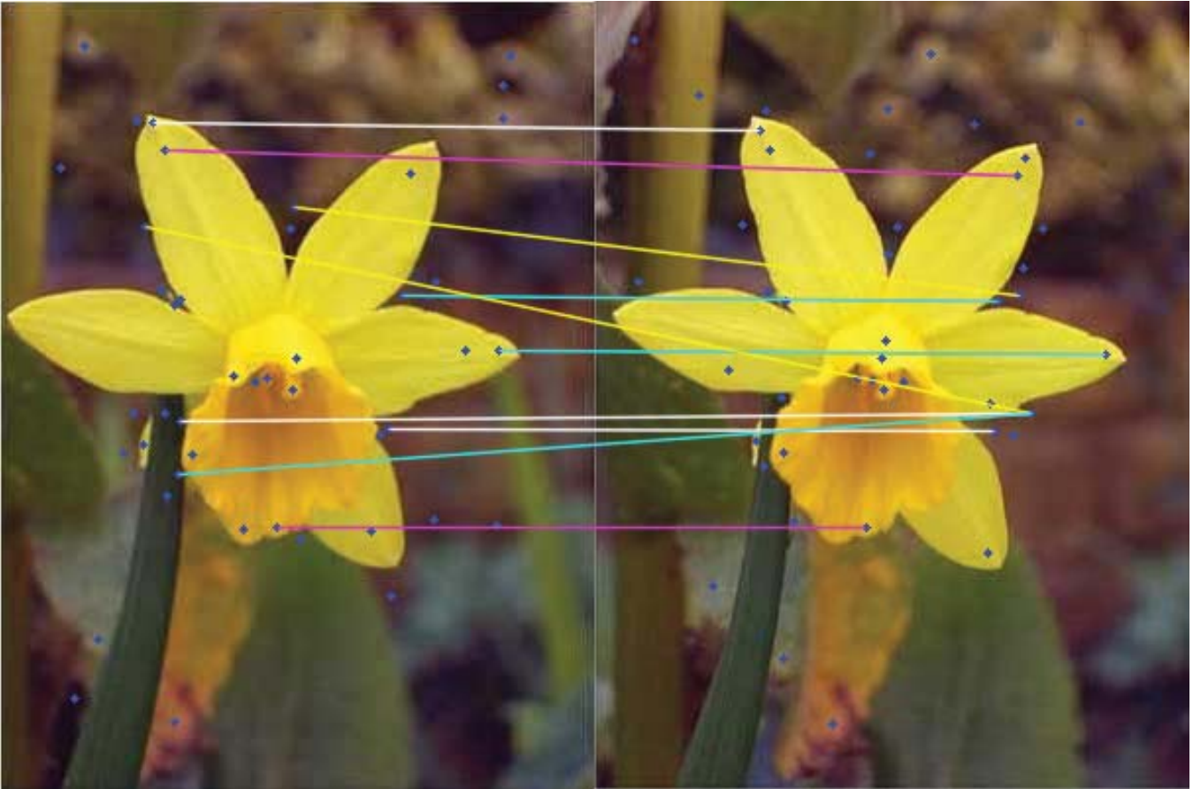
Figure 11: SURF on stereo.jpg, stereo1.jpg - 10 correspondences found but lots of false positives
