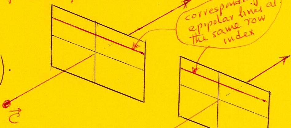
Pretend for a moment that the epipole in the right image is at  $(f, 0, 1)^T$ . It is easy to show that the homography  $G = \begin{bmatrix} * & 0 & 0 \\ 0 & 1 & 0 \\ -1/f & 0 & 1 \end{bmatrix}$  will take that epipole to  $\begin{pmatrix} 1 \\ 0 \\ 0 \end{pmatrix}$ .
