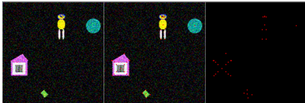
(a) An image, the image with keypoints superimposed, and just the keypoints
