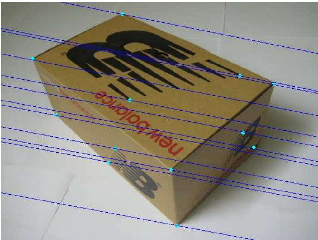
Figure 2. Manually selected 12 point pairs and the estimated epipolar lines
