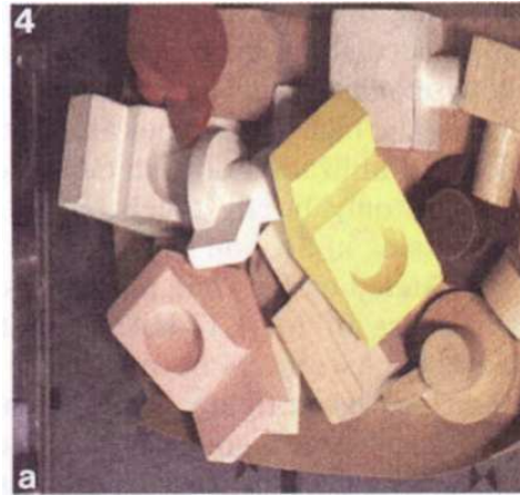
Figure 28: The yellow and the white objects shown in this pile were used for demonstrating the dependence of the measured color on the orientation of a surface.
