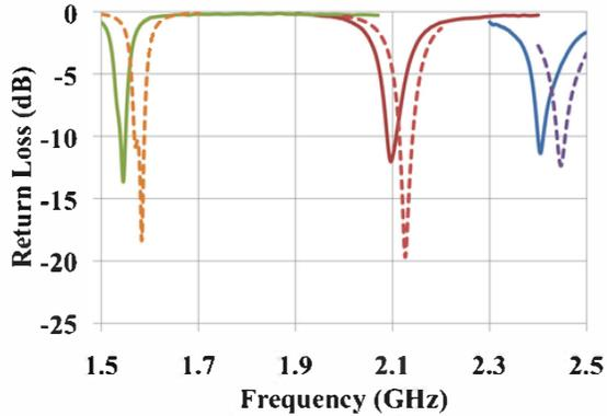
Fig. 4 Measured (solid line) and simulated (dashed line) return loss.
