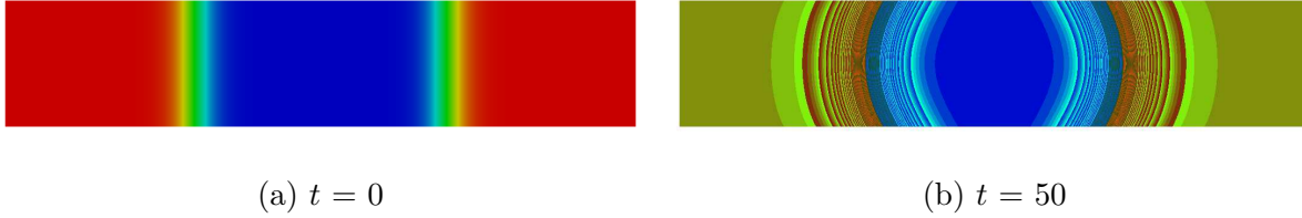
Figure 4: Density field ( \rho ) at t = 0 and t = 50 obtained from the Navier-Stokes-Korteweg equations (6). The results are computed using the proposed method with p = 3 and h = 2^{-6} .
